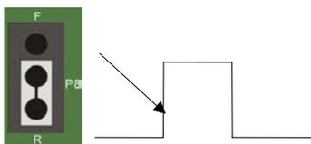
Figure 5. Jumper P8 set for rising edge
