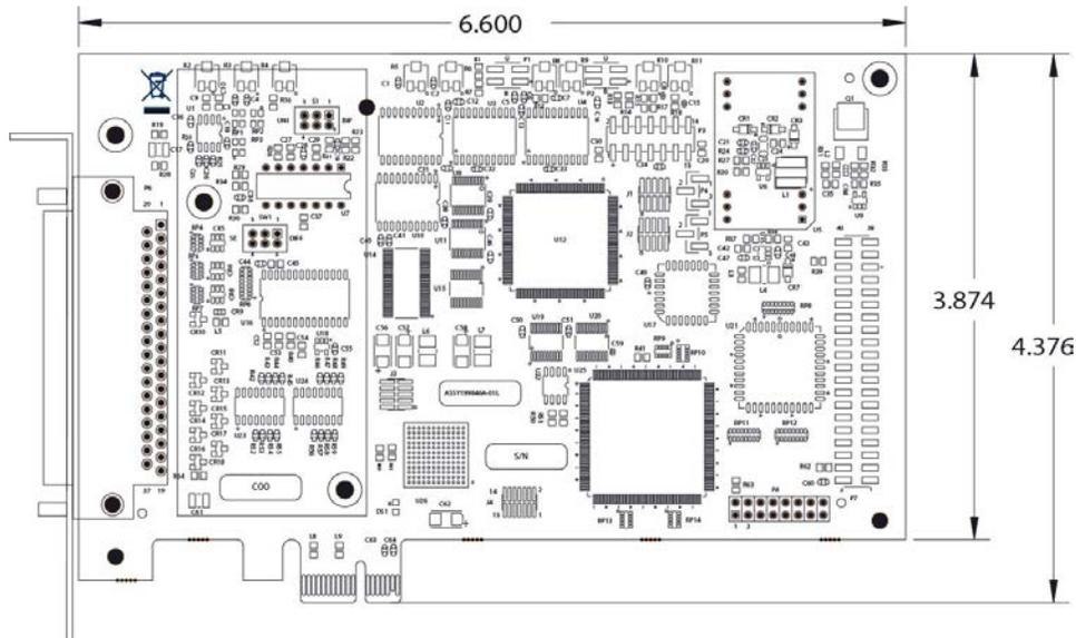
Figure 17. PCIe-DAS1602/16 circuit board dimensions (inches)
