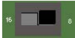
Figure 3. 16/8 channel select switch (S1) default setting (8)
