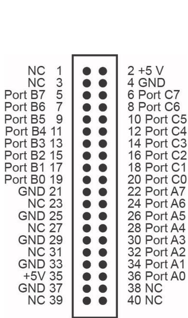
Figure 12. Digital I/O connector pin out
