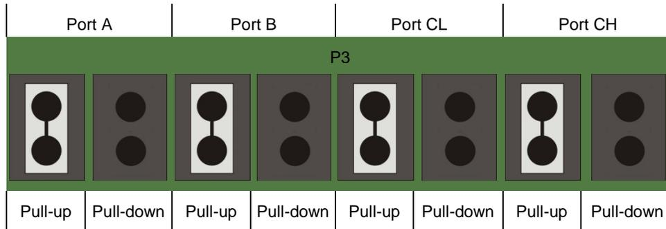
Figure 10. Pull-up/pull-down jumpers (P3)
