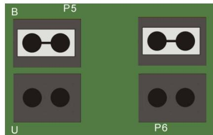
Figure 8. DAC0 (P5) and DAC1 (P6) unipolar/bipolar jumpers
