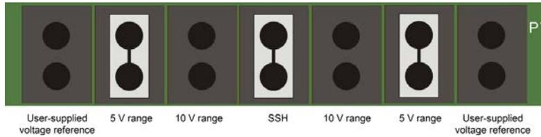
Figure 7. DAC0 and DAC1 range jumpers (P7)
