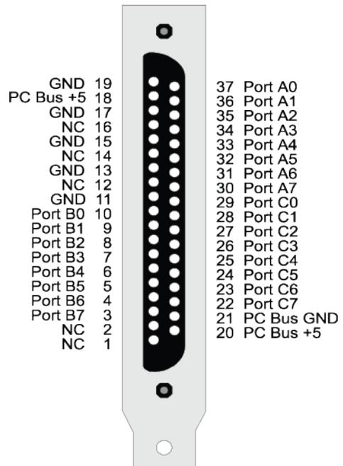
Figure 13. BP40-37 connector pin out
