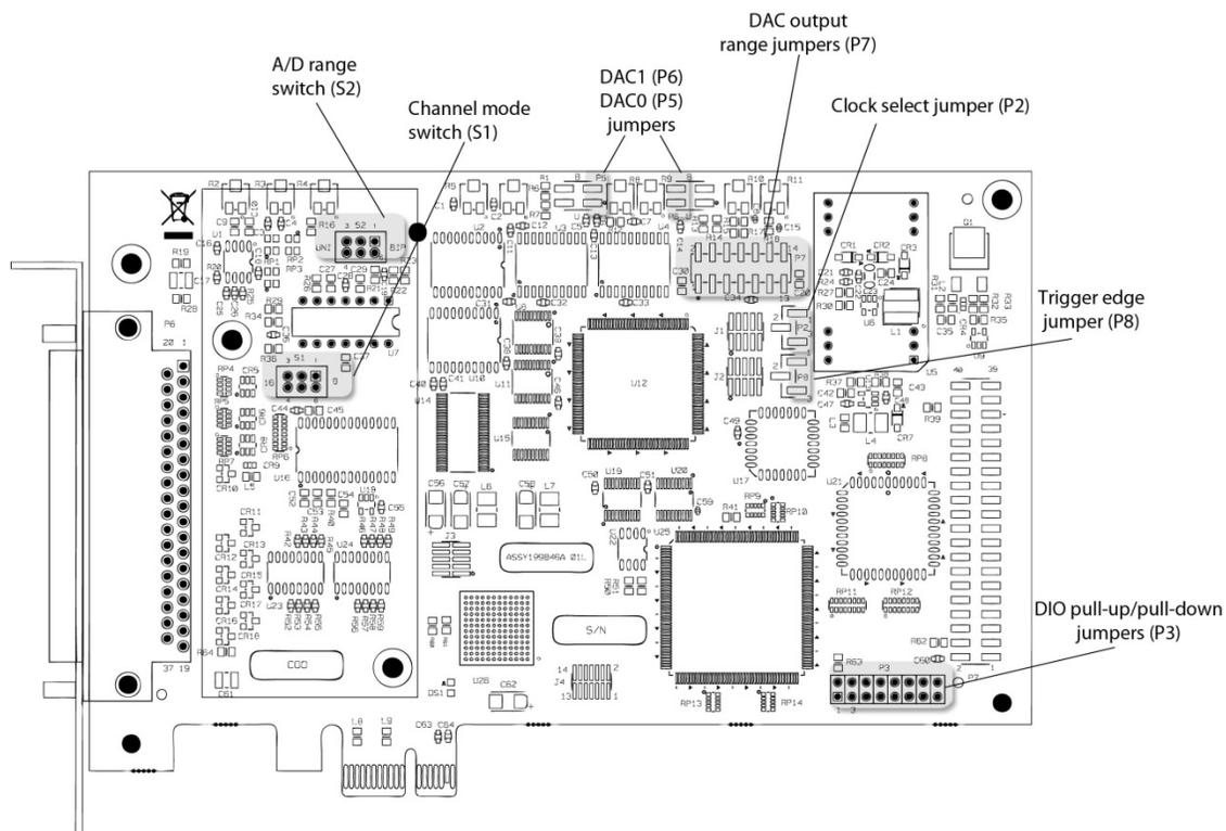
Figure 2. PCIe-DAS1602/16 switch and jumper locations
