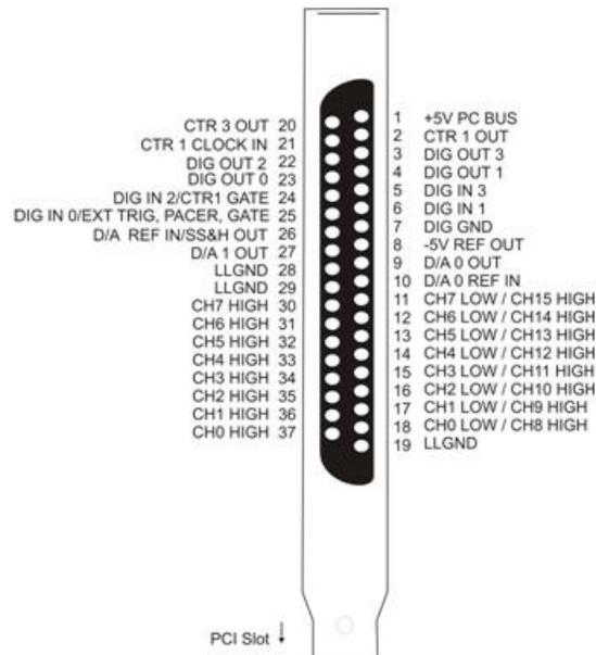
Figure 11. Main I/O connector pin out
