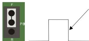
Figure 6. Jumper P8 set for falling edge
