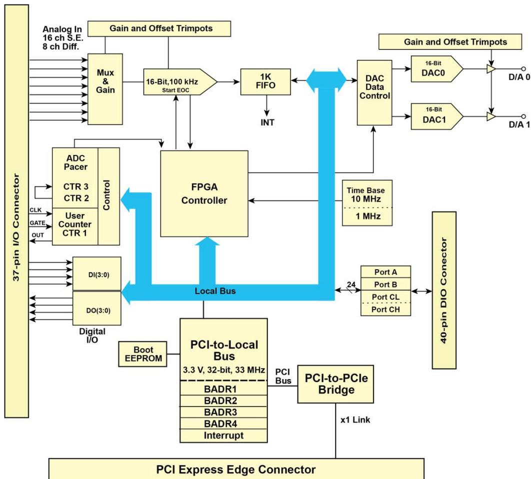
Figure 1. PCIe-DAS1602/16 functional block diagram
