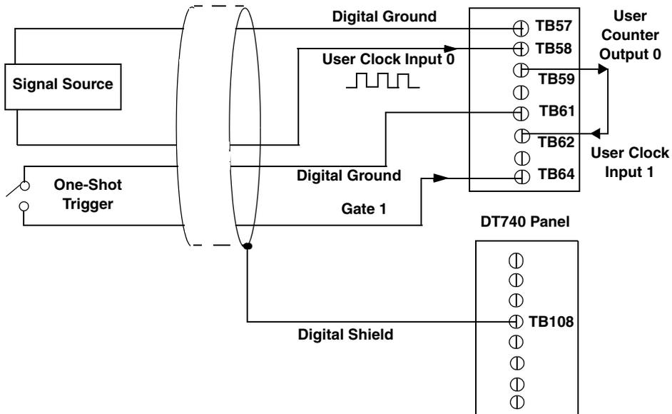
**Figure 48: Cascading Counters for the DT740**
