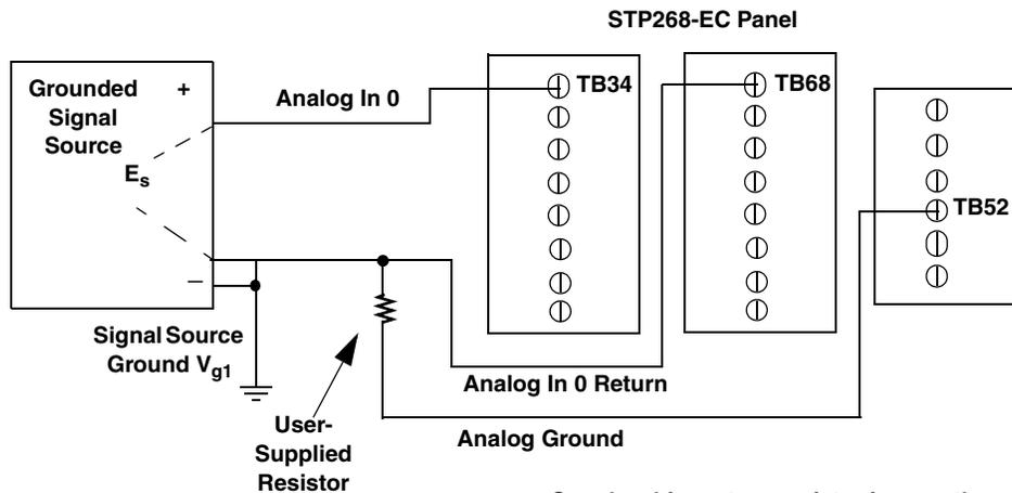
Supply a bias return resistor in case the external ground is floating.
