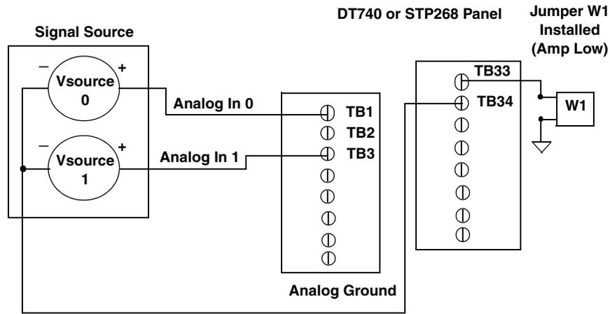
Note that the signals shown for the STP268 screw terminal panel correspond to connector J1.
