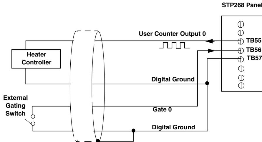
Note that the signals shown for the STP268 screw terminal panel correspond to connector J1.
