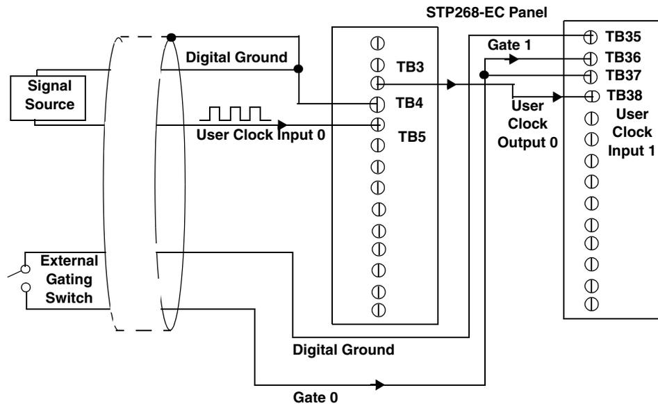
Note that you can internally cascade counters using software; if you internally cascade the counters, you do not have to make the external cascading connections. Note also that this example shows the use of an external gate; however, this connection is not required.
