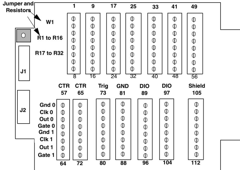
Figure 12: Layout of the DT740 Screw Terminal Panel
