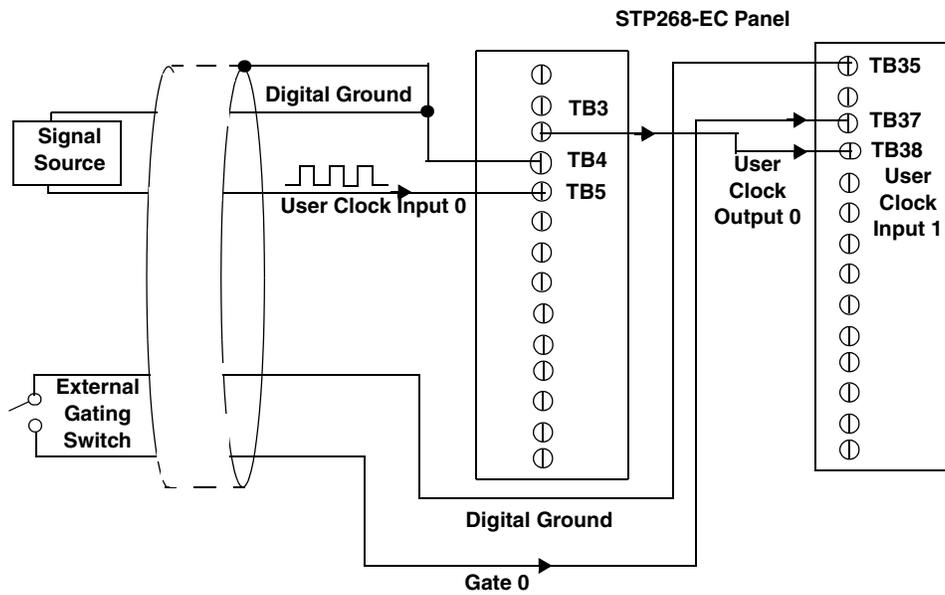
**Figure 53: Cascading Counters to the STP268-EC**
