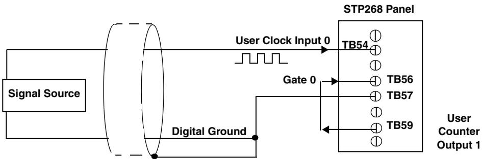
Note that the signals shown for the STP268 screw terminal panel correspond to connector J1.
