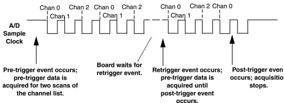
**Figure 60: Continuous Pre-Trigger Mode with Triggered Scan**
