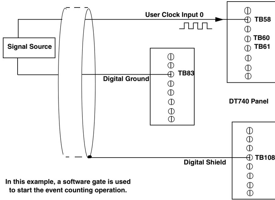
**Figure 35: Connecting Event Counting Applications to the DT740
