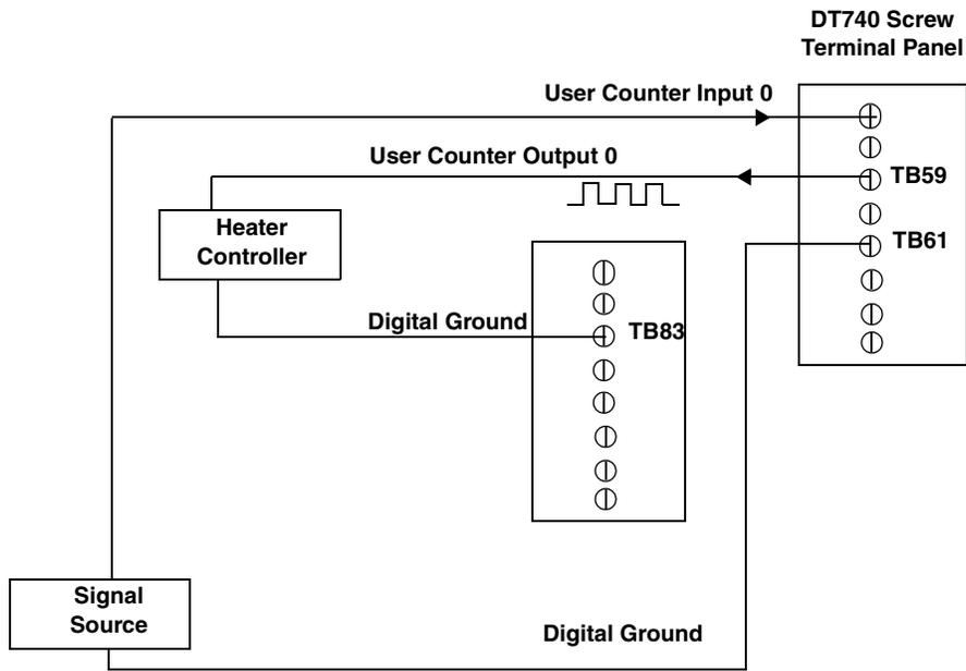
**Figure 70: Connecting Rate Generation Signals
