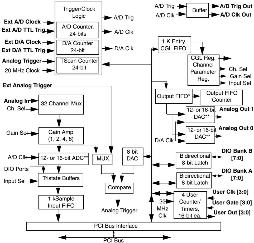
\*The DT3010, DT3010-268, and DT3016 have a 4 kSample output FIFO; the DT3010/32 and DT3010/32-268 have a 32 kSample output FIFO.\*\*Only the DT3016 has a 16-bit ADC and 16-bit DACs.
