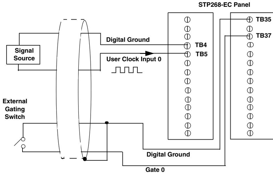
In this example, rising clock edges are counted while the gate is active.
