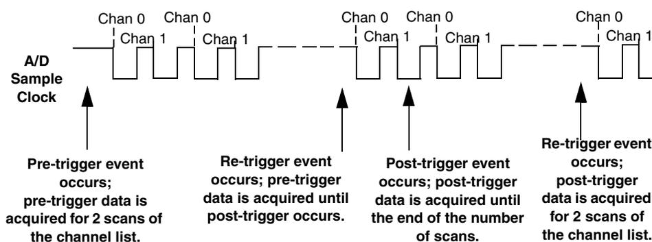
**Figure 62: Continuous About-Trigger Mode with Triggered Scan**
