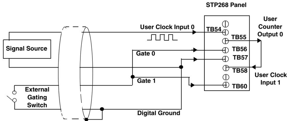
Note that the signals shown for the STP268 screw terminal panel correspond to connector J1.
