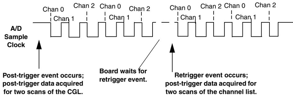
**Figure 58: Continuous Post-Trigger Mode with Triggered Scan**
