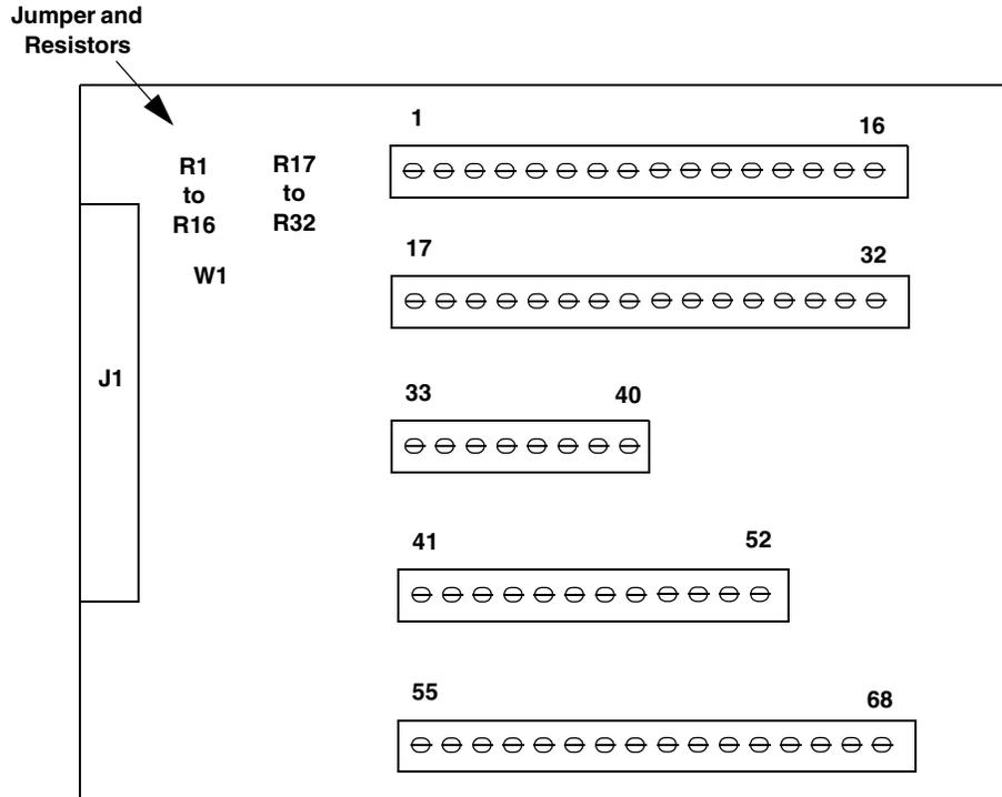
**Figure 13: Layout of the STP268 Screw Terminal Panel**
