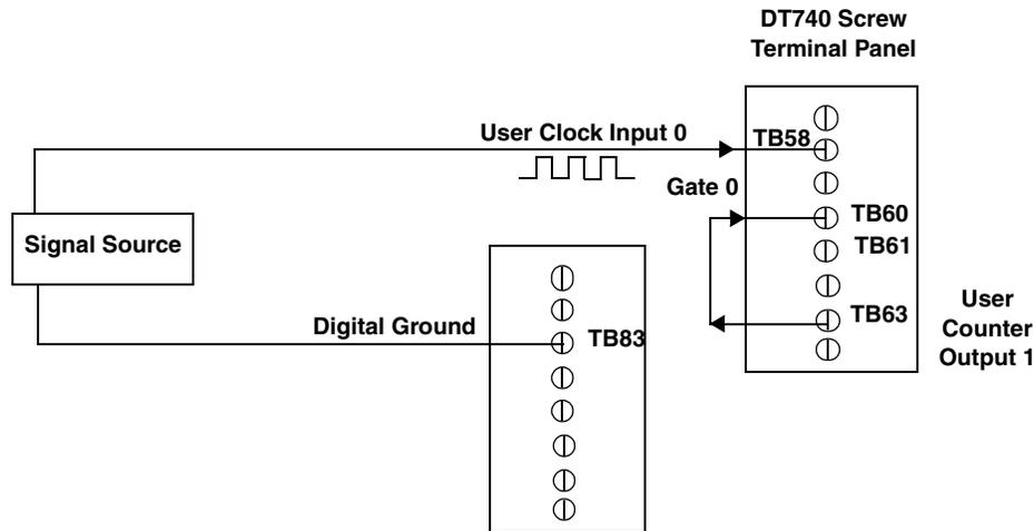
**Figure 68: Connecting Frequency Measurement Signals
