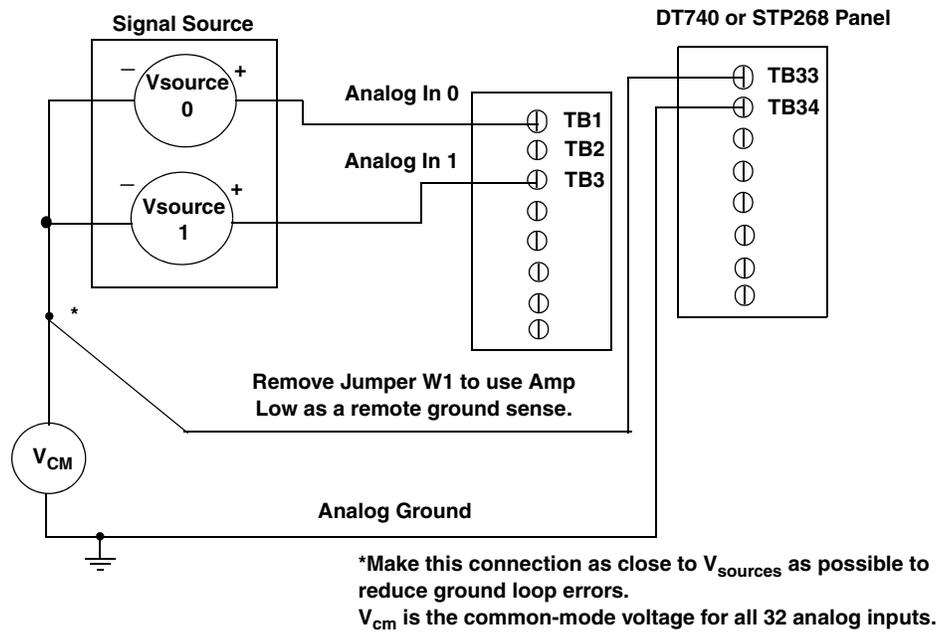
Note that the signals shown for the STP268 screw terminal panel correspond to connector J1.
