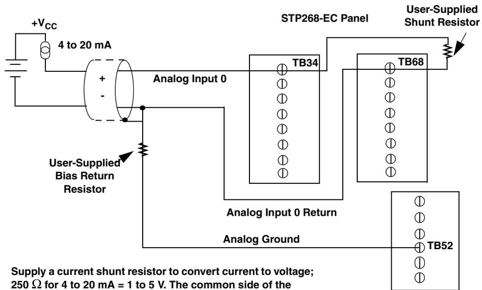
Supply a current shunt resistor to convert current to voltage; 250  $\Omega$  for 4 to 20 mA = 1 to 5 V. The common side of the external loop supply must either connect to analog ground or, if needed, to a bias return resistor.
