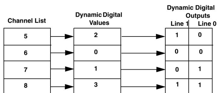
**Figure 56: An Example Using Dynamic Digital Outputs**
