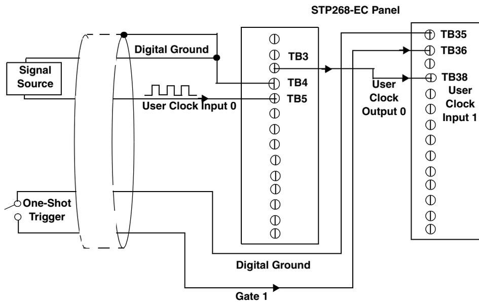
**Figure 54: Cascading Counters for the STP268-EC**
