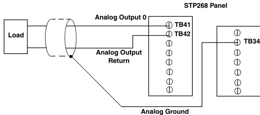
Note that the signals shown for the STP268 screw terminal panel correspond to connector J1.
