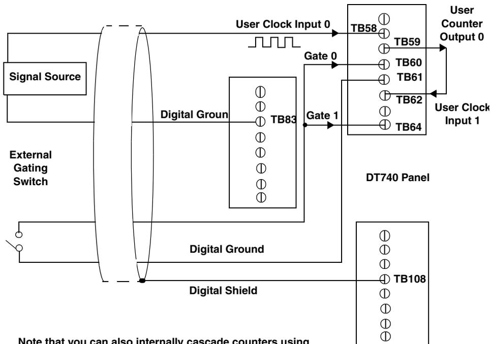
Note that you can also internally cascade counters using software; if you internally cascade the counters, you do not have to make the external cascading connections. Note also that this example shows the use of an external gate; however, this connection is not required.
