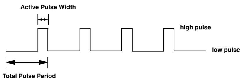
Figure 64: Example of a Low-to-High Pulse Output Type
