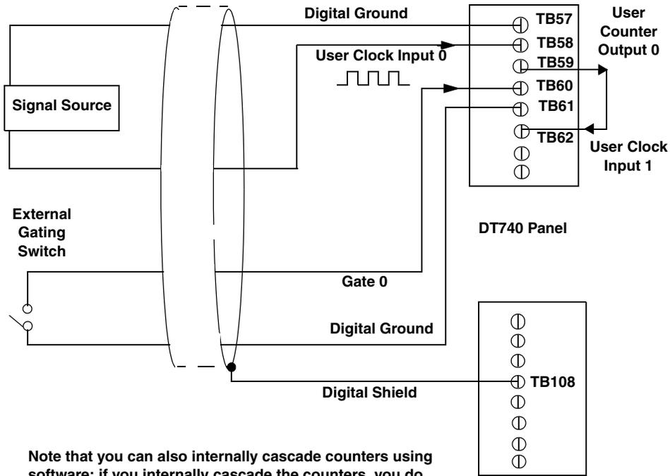
Note that you can also internally cascade counters using software; if you internally cascade the counters, you do not have to make the external cascading connections. In this example, counter 1 gate is logic high.
