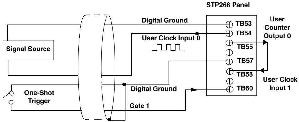
Note that the signals shown for the STP268 screw terminal panel correspond to connector J1.
