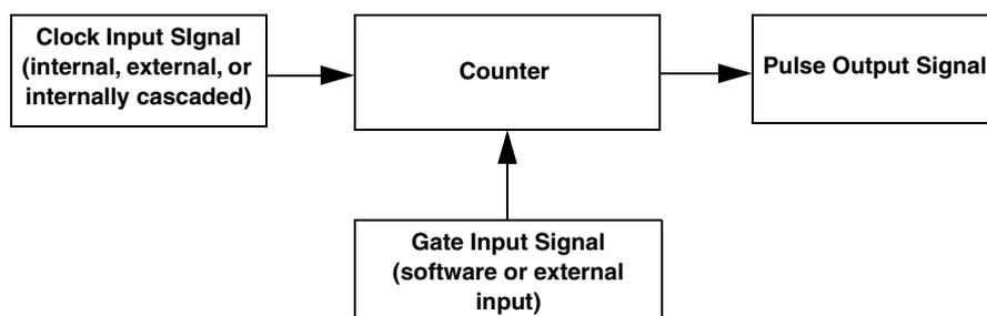
**Figure 63: Counter/Timer Channel**
