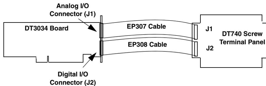
Figure 3: Attaching the DT740 Screw Terminal Panel to the DT3034 Board
