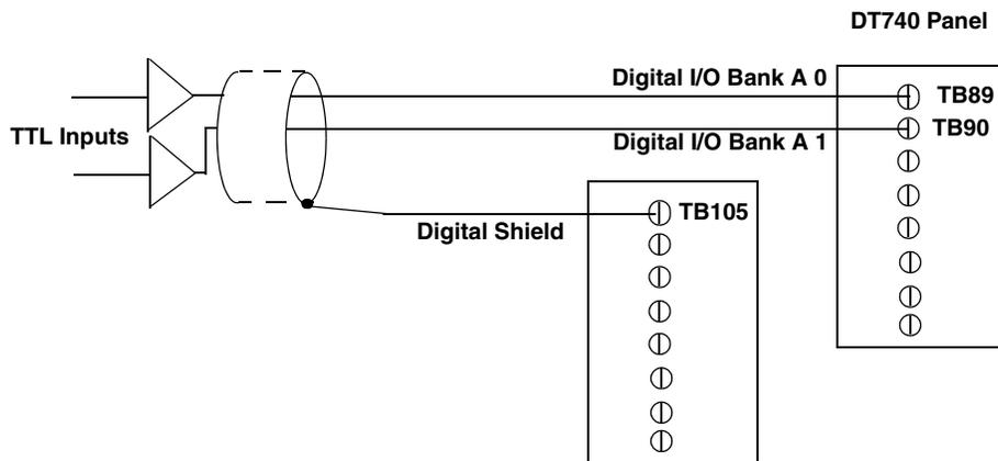
**Figure 11: Connecting Digital Inputs to the DT740 (Shown for Lines 0 and 1, Bank A)**
