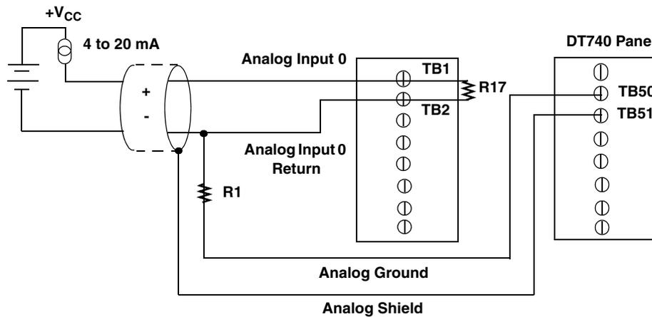
Use current shunt resistor R17 to convert current to voltage;  $250\ \Omega$  for 4 to 20 mA = 1 to 5 V. The common side of the external loop supply must either connect to analog ground or, if needed, to a bias return resistor (R1 in this case).
