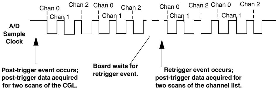
**Figure 23: Continuous Post-Trigger Mode with Triggered Scan**
