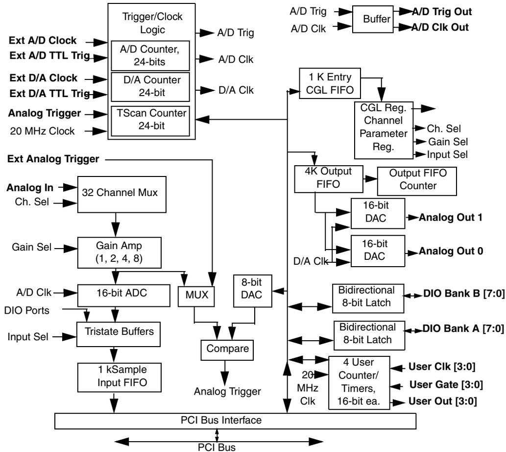
**Figure 20: Block Diagram of the DT3034 Board**
