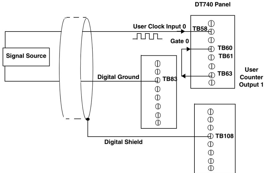
**Figure 16: Connecting Frequency Measurement Applications to the DT740 Screw Terminal Panel (Shown for Clock Input 0 and External Gate 0)**
