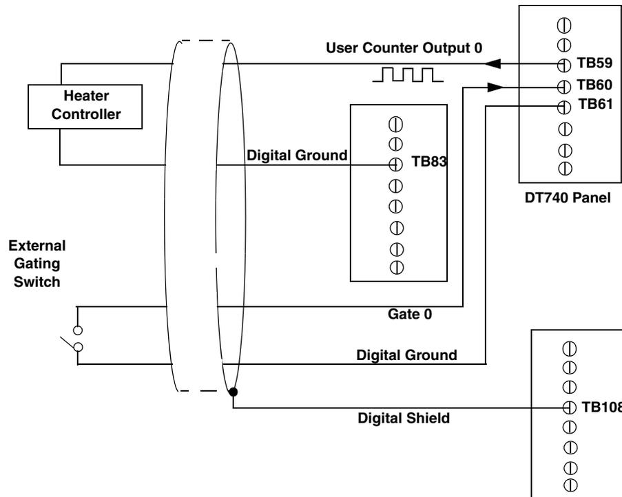
Figure 17: Connecting Pulse Output Applications to the DT740 Screw Terminal Panel (Shown for Counter Output 0 and Gate 0)
