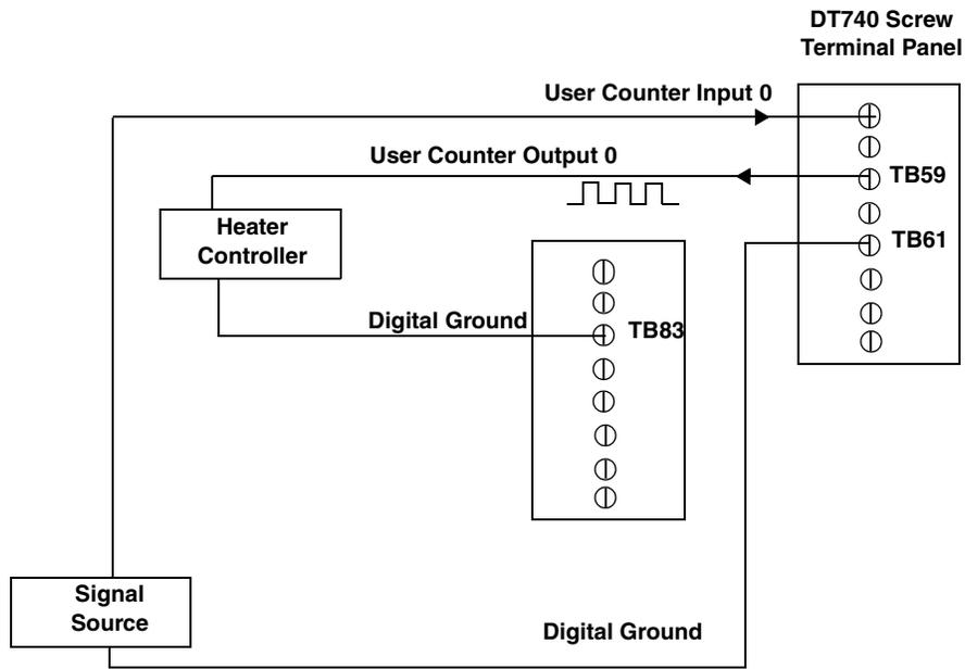
**Figure 34: Connecting Rate Generation Signals
