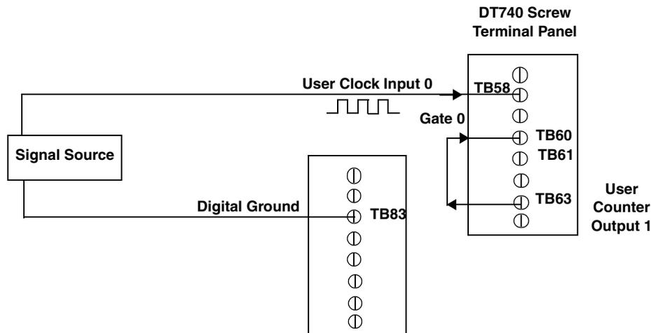
**Figure 32: Connecting Frequency Measurement Signals
