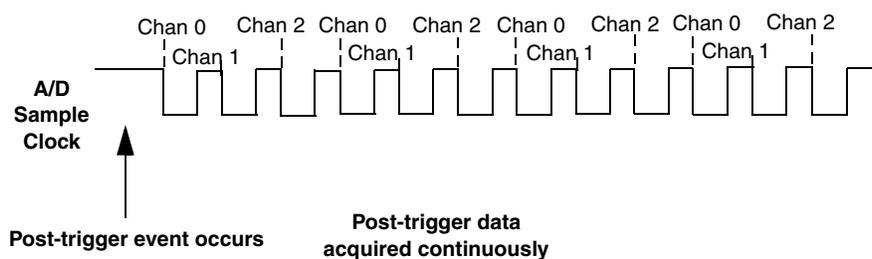
**Figure 22: Continuous Post-Trigger Mode without Triggered Scan**
