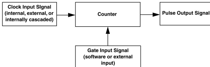
**Figure 28: Counter/Timer Channel**
