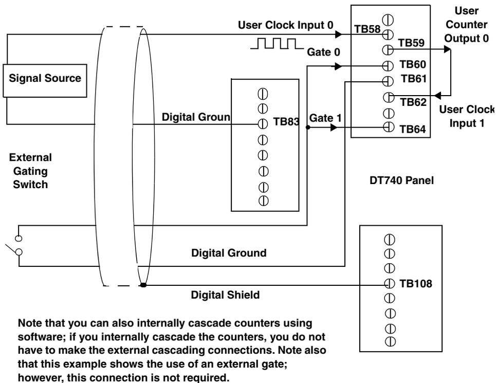
**Figure 15: Cascading Counters on a DT740 Screw Terminal Panel (Shown for Event Counting Using Counters 0 and 1 and External Gate 0)**
