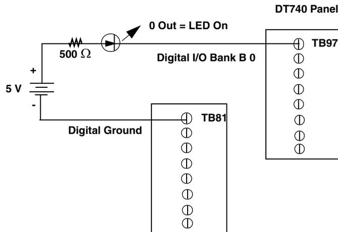
**Figure 12: Connecting Digital Outputs to the DT740 (Shown for Line 0, Bank B)**
