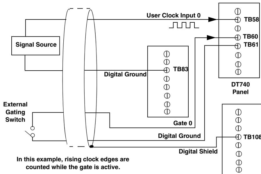
**Figure 13: Connecting Event Counting Applications to the DT740 (Shown for Clock Input 0 and an External Gate 0)**
