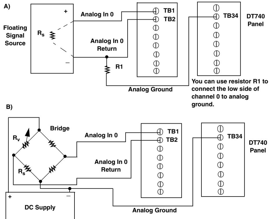
**Figure 7: Connecting Differential Voltage Inputs to the DT740 (Shown for Channel 0)**
