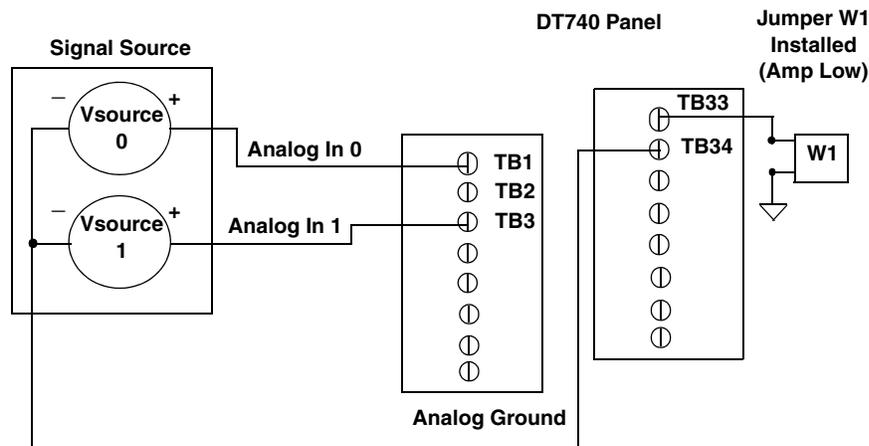
**Figure 5: Connecting Single-Ended Voltage Inputs to the DT740 (Shown for Channels 0 and 1)**
