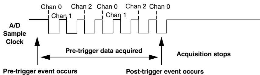
**Figure 24: Continuous Pre-Trigger Mode**
