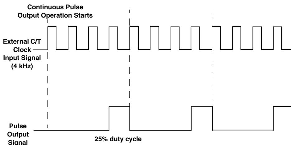
**Figure 36: Example of Rate Generation Mode with a 25% Duty Cycle**
