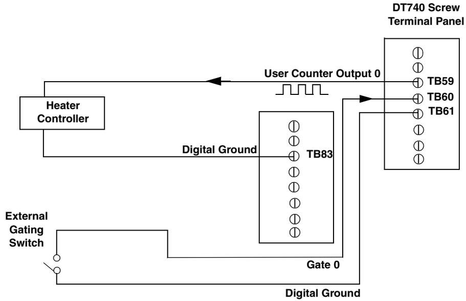
**Figure 37: Connecting One-Shot Signals (Shown for Counter Output 0 and Gate 0)**
