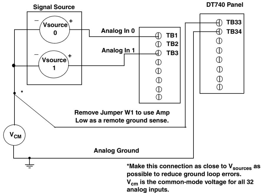
Figure 6: Connecting Pseudo-Differential Voltage Inputs to the DT740 (Shown for Channels 0 and 1)
