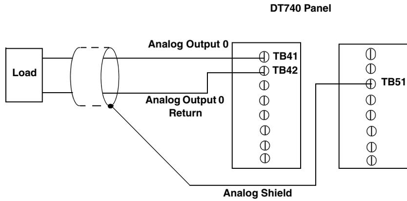
Figure 10: Connecting Analog Output Voltages to the DT740 (Shown for Channel 0)
