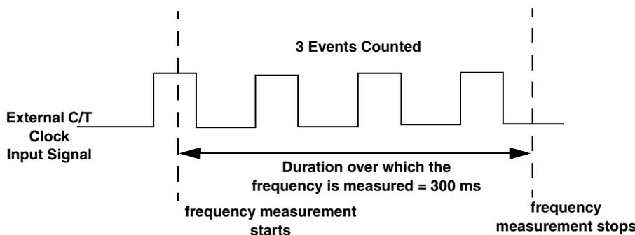
Figure 33: Example of Frequency Measurement
