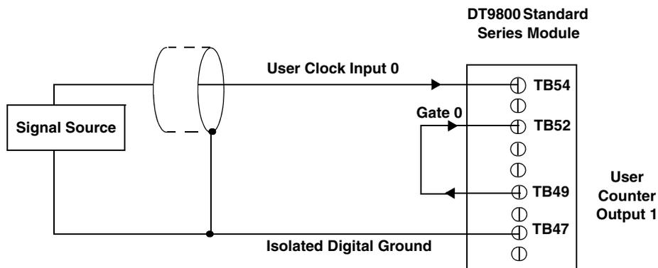
**Figure 24: Connecting Frequency Measurement Signals
