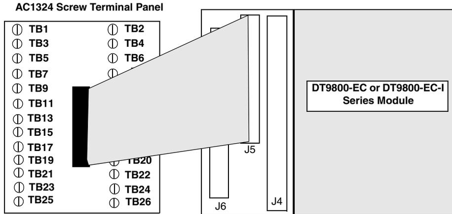
**Figure 39: Attaching the AC1324 Screw Terminal Panel to Connector J5 of the DT9800-EC/EC-I Series for +5 V Power**
