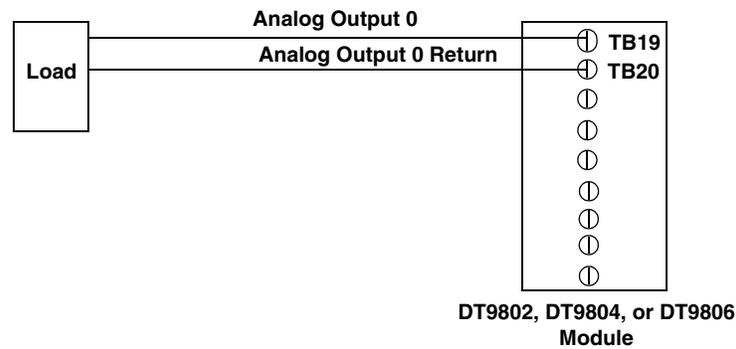
Figure 18: Connecting Analog Output Voltages (Shown for Channel 0)
