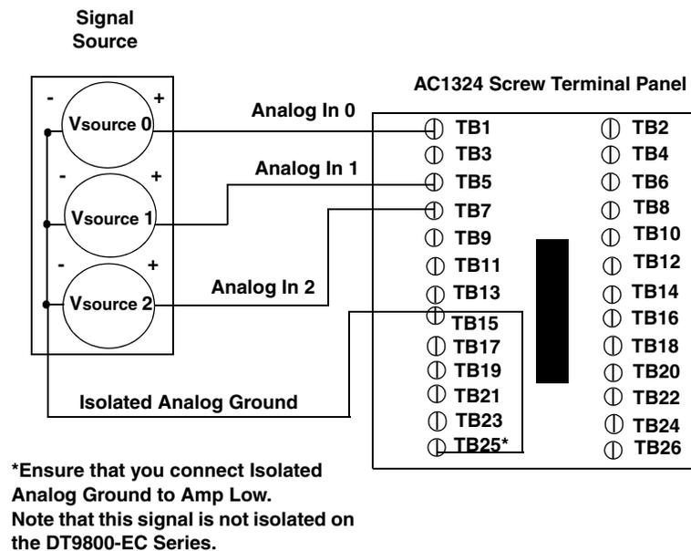
**Figure 29: Connecting Single-Ended Voltage Inputs
