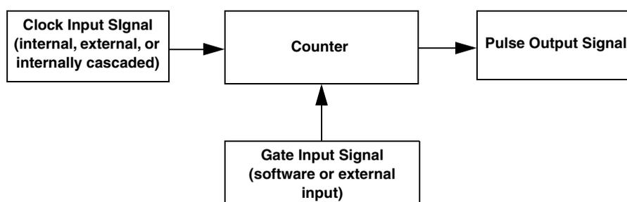
**Figure 53: Counter/Timer Channel**
