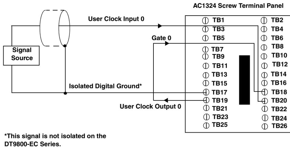
**Figure 45: Connecting Frequency Measurement Signals
