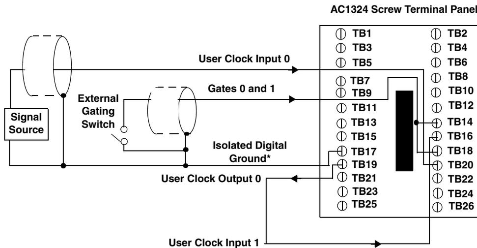
**Figure 44: Cascading Counters (Shown for Event Counting Using Counters 0 and 1 and External Gate 0)**
