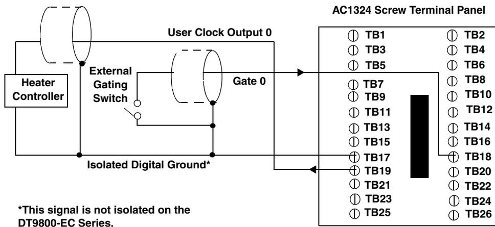
**Figure 46: Connecting Pulse Output Signals
