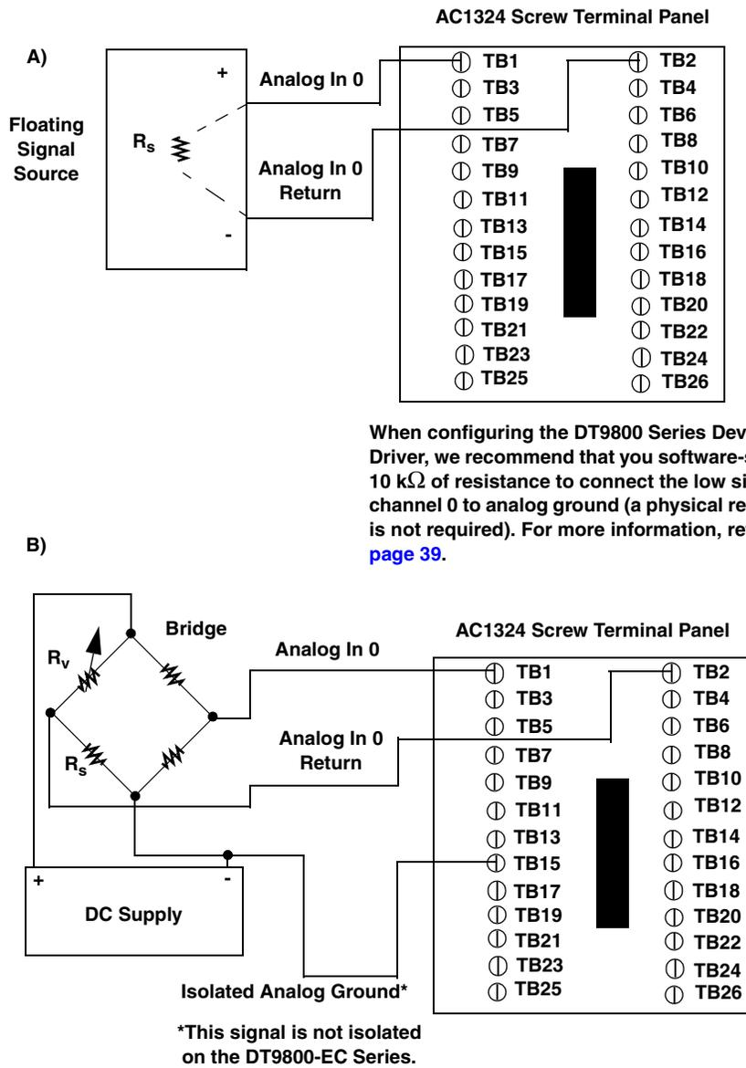
**Figure 31: Connecting Differential Voltage Inputs (Shown for Channel 0)**
