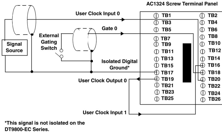
**Figure 47: Cascading Counters (Shown for Rate Generation Using Counters 0 and 1 and External Gate 0)**
