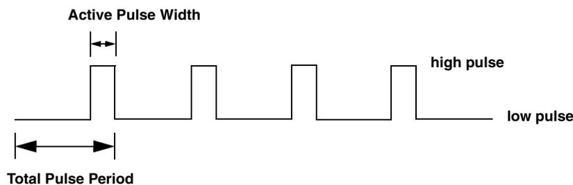
**Figure 54: Example of a Low-to-High Pulse Output Type**
