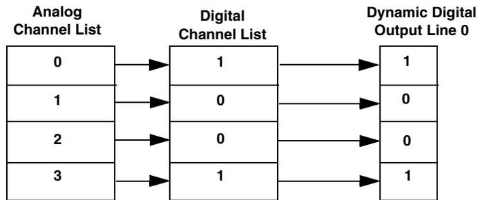
**Figure 50: An Example Using Dynamic Digital Outputs**
