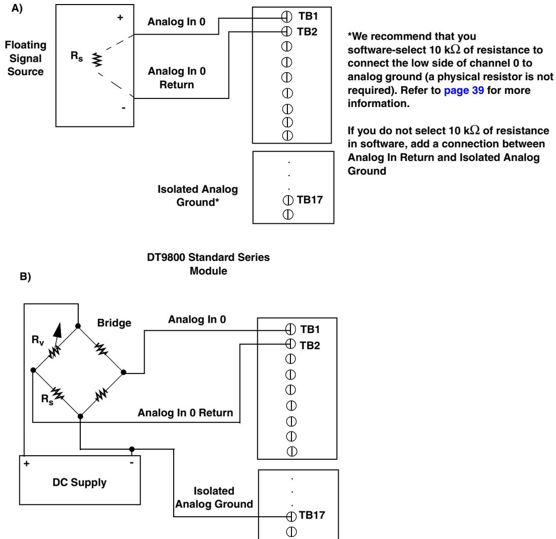
**Figure 14: Connecting Differential Voltage Inputs (Shown for Channel 0)**
