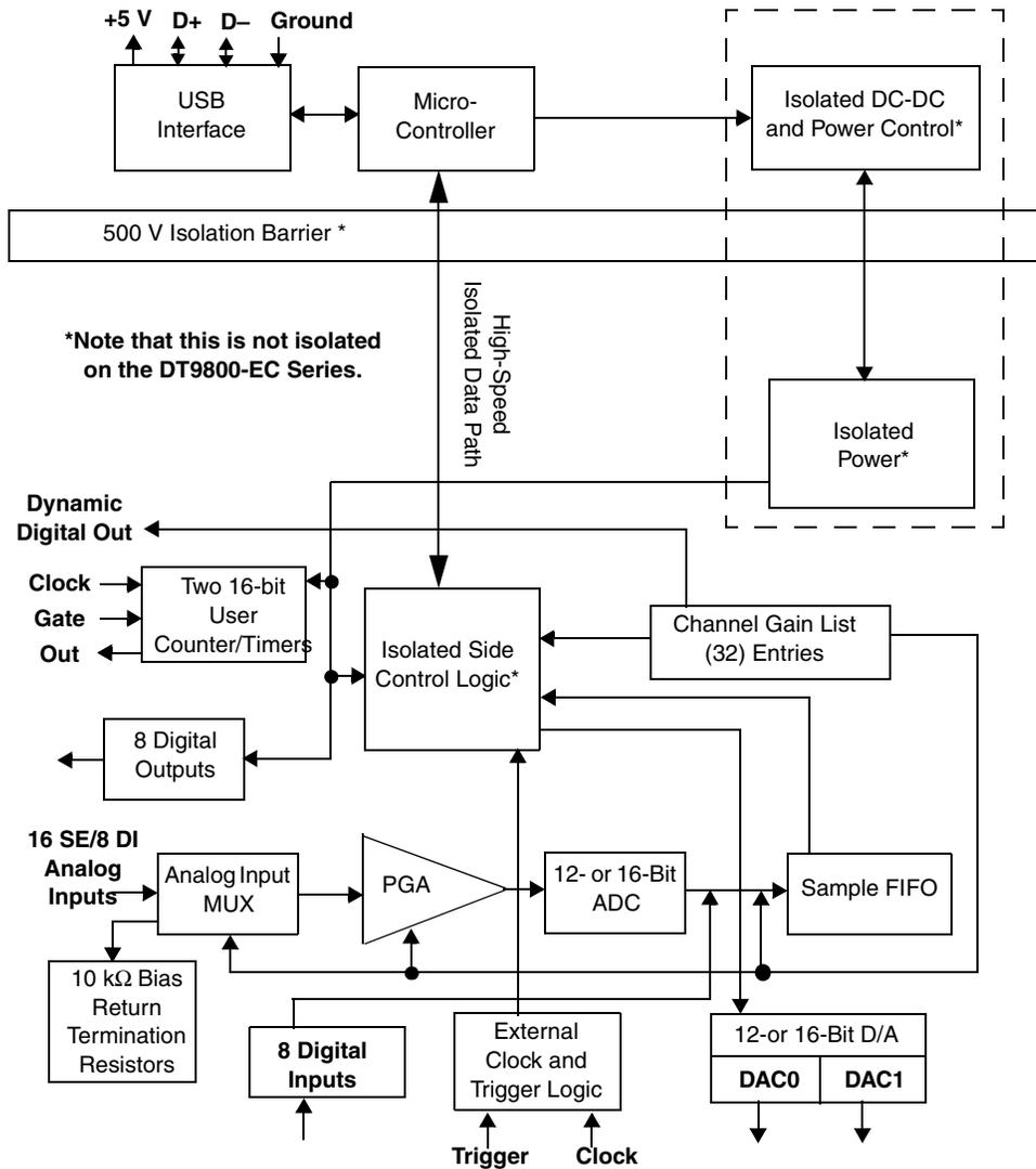
Figure 49: Block Diagram of the DT9800 Series Modules
