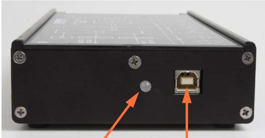
The USB LED is green when the module is powered and blinks amber when the module is acquiring data.
