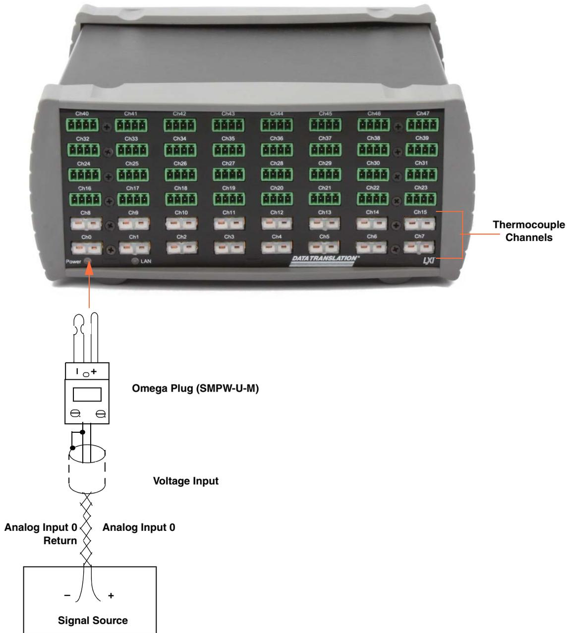
Figure 20: Connecting Voltage Inputs to a Thermocouple Channel
