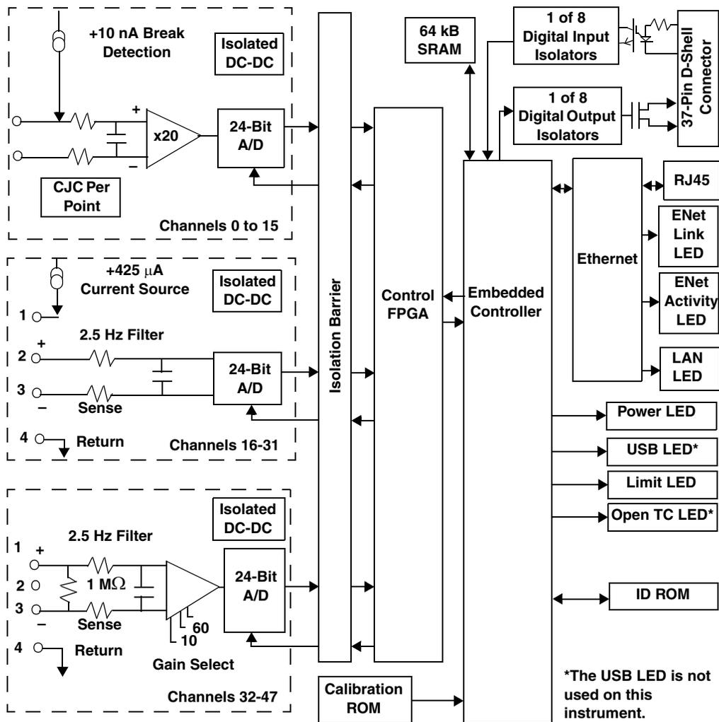
Figure 36: Block Diagram of the DT8874 MEASURpoint Instrument
