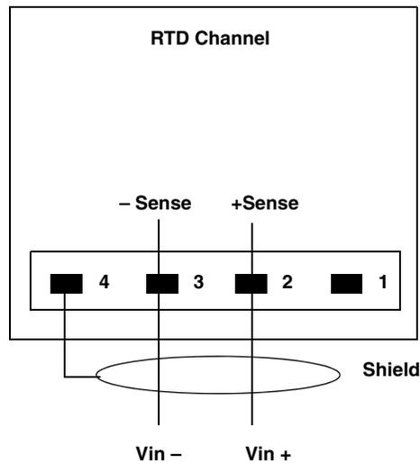
**Figure 21: Connecting Voltage Inputs to an RTD Channel**
