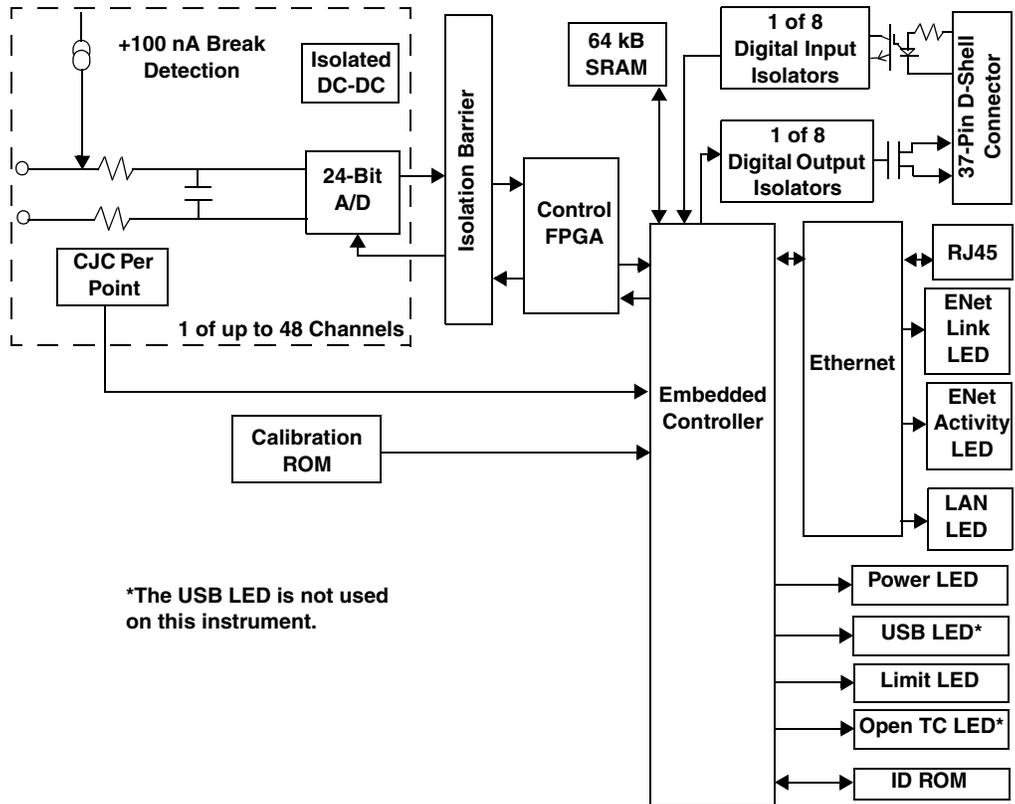
Figure 33: Block Diagram of the DT8871 TEMPpoint Instrument
