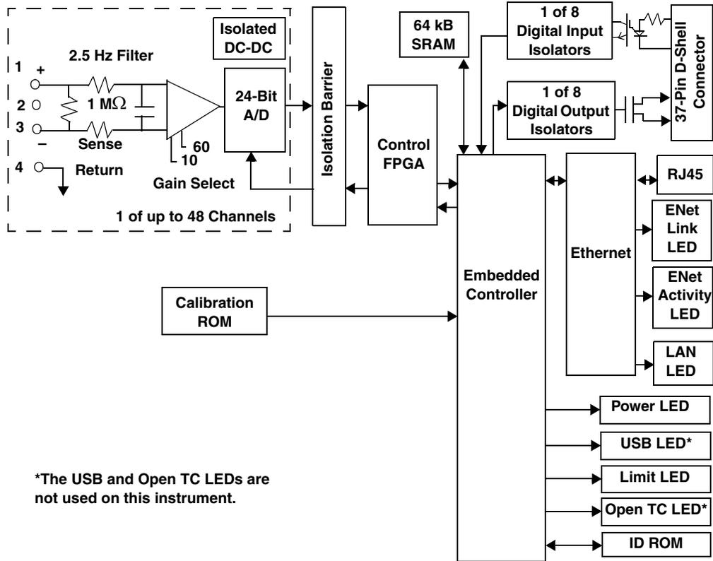
Figure 35: Block Diagram of the DT8873 VOLTpoint Instrument
