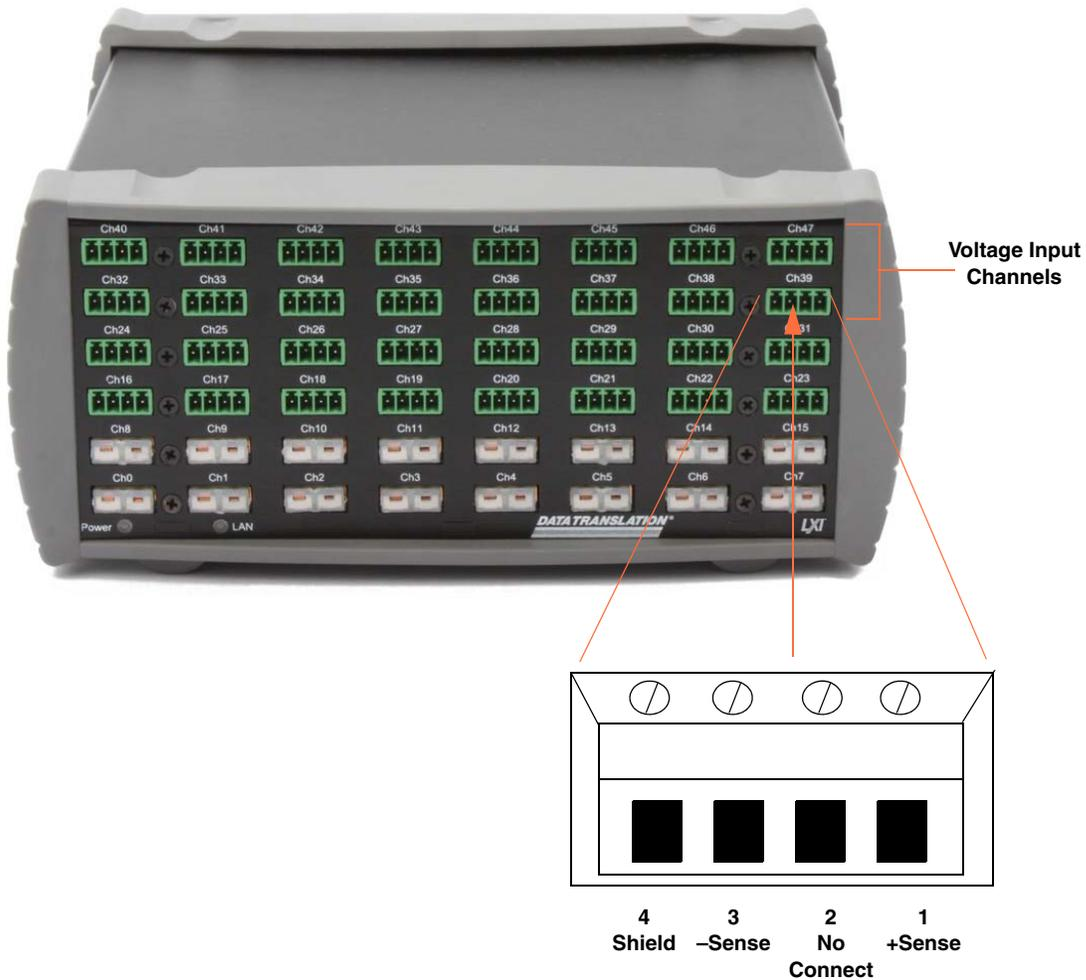
**Figure 22: Screw Terminal Block Numbering for Voltage Connections**
