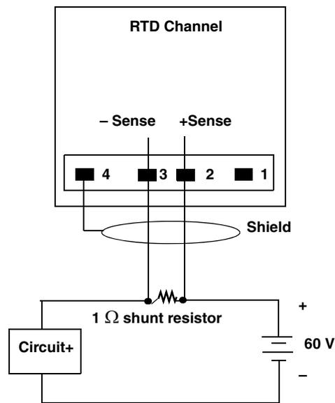
Use a  $1\ \Omega$  shunt resistor to convert current to voltage:  $1\ \Omega = 1.25\ \text{A} = 1.25\ \text{V}$ .
