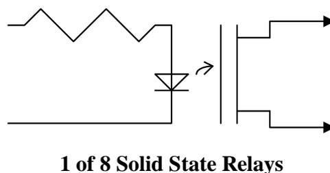
**Figure 39: Digital Output Circuitry**
