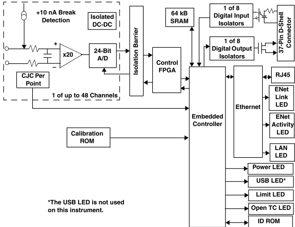
Figure 32: Block Diagram of the DT8871U TEMPpoint Instrument
