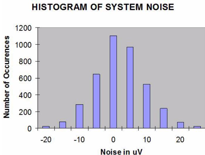
Figure 42: System Noise on the DT8871 Using No Software Filter (Raw Filter)
