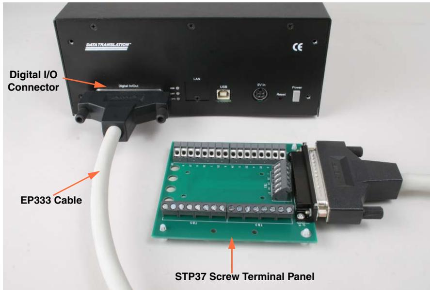
**Figure 27: Connecting the Instrument to the STP37**
