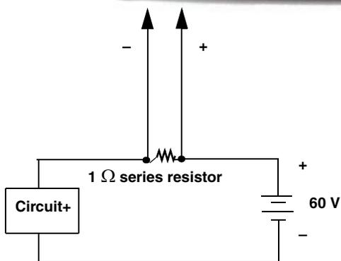
Use a 1  $\Omega$  series resistor to convert current to voltage.
