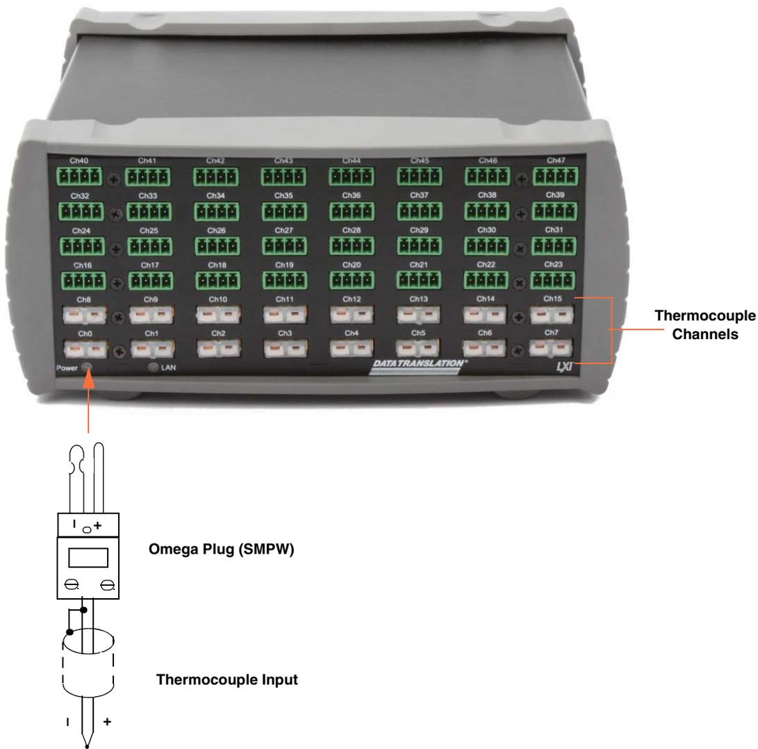
**Figure 15: Connecting Thermocouple Inputs**
