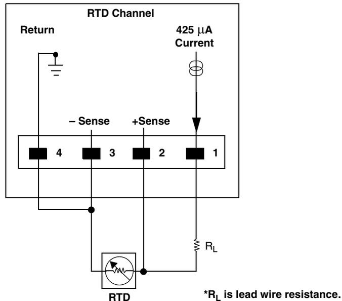
Figure 18: 3-Wire RTD Connection
