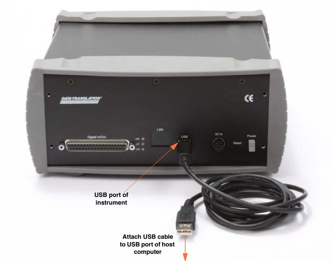
**Figure 9: Attaching the Instrument to the Host Computer**
