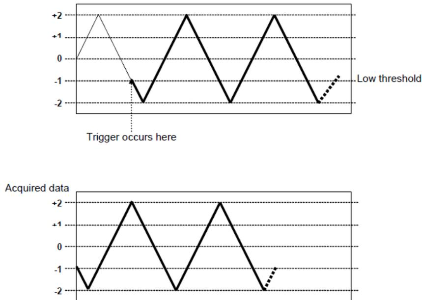
Figure 14. Trigger below, edge-sensitive
