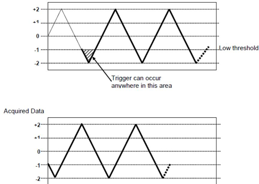
Figure 12. Trigger below, level-sensitive
