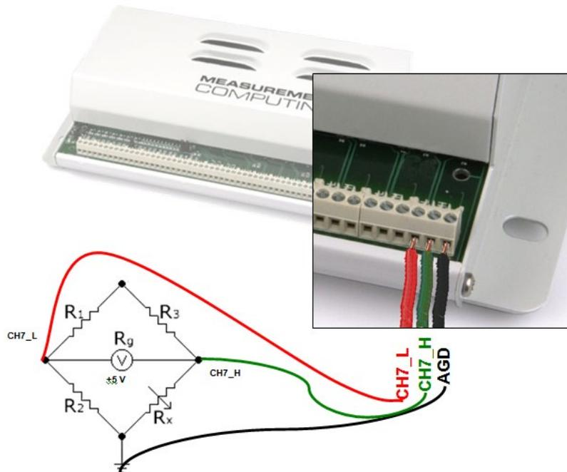
Figure 7. Differential measurement connection
