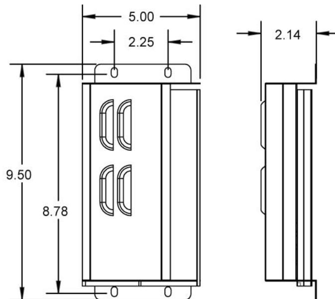
Figure 10. USB-1616FS enclosure dimensions
