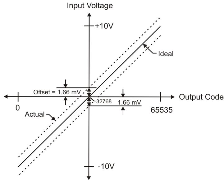
Figure 6. USB-1616FS transfer function with offset error
