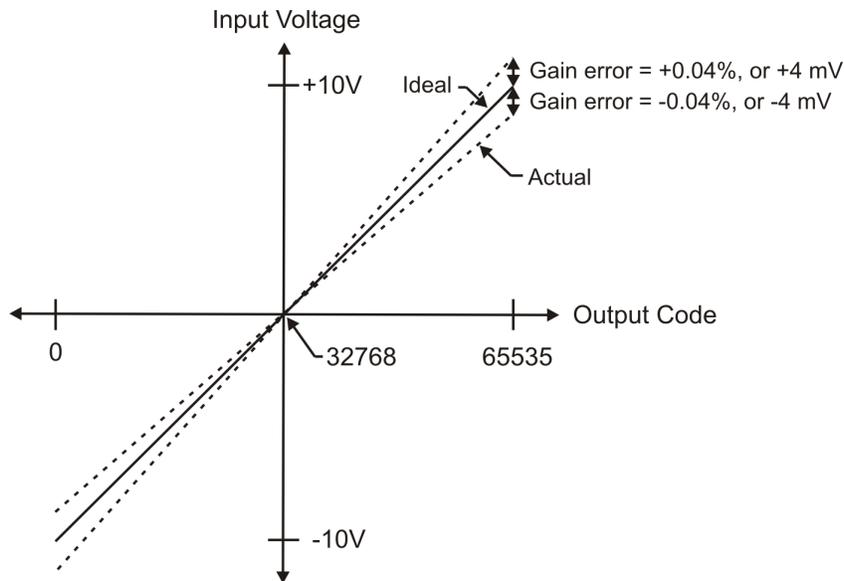
Figure 7. USB-1616FS transfer function with gain error
