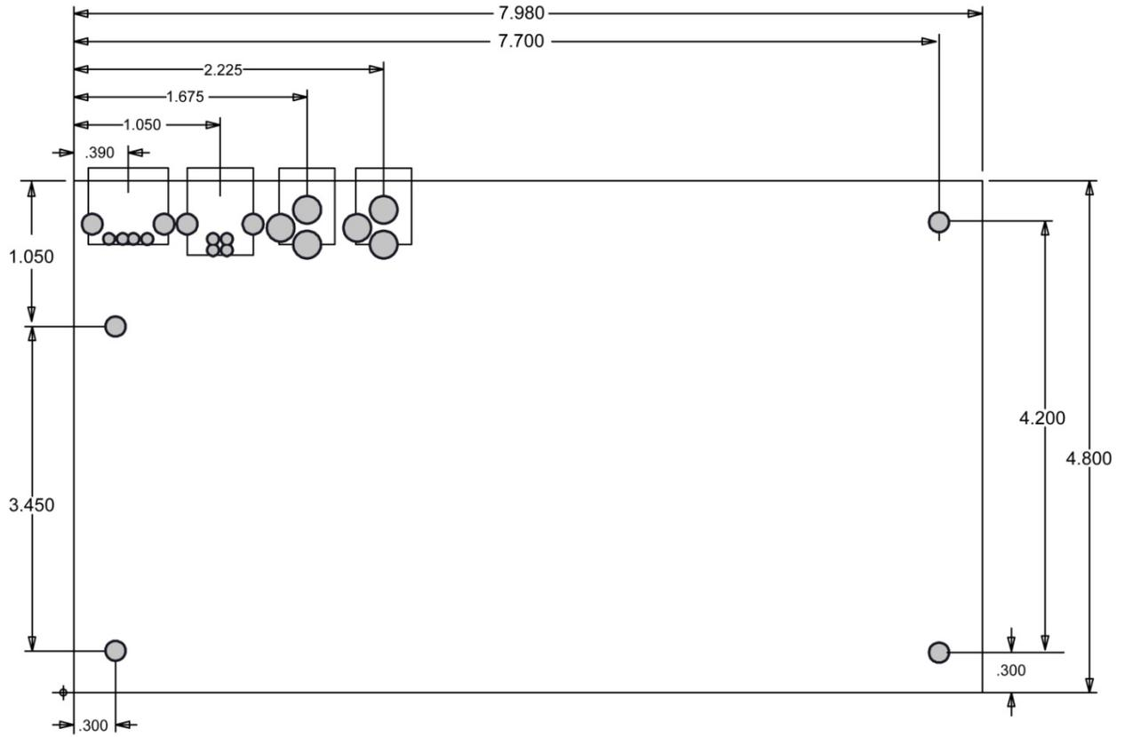
Figure 9. USB-1616FS circuit board dimensions
