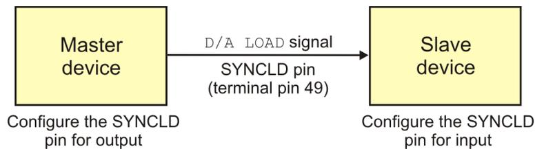
Figure 8. Synchronizing the update of multiple units
