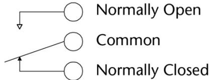
Figure 4. Form C SPDT relay
