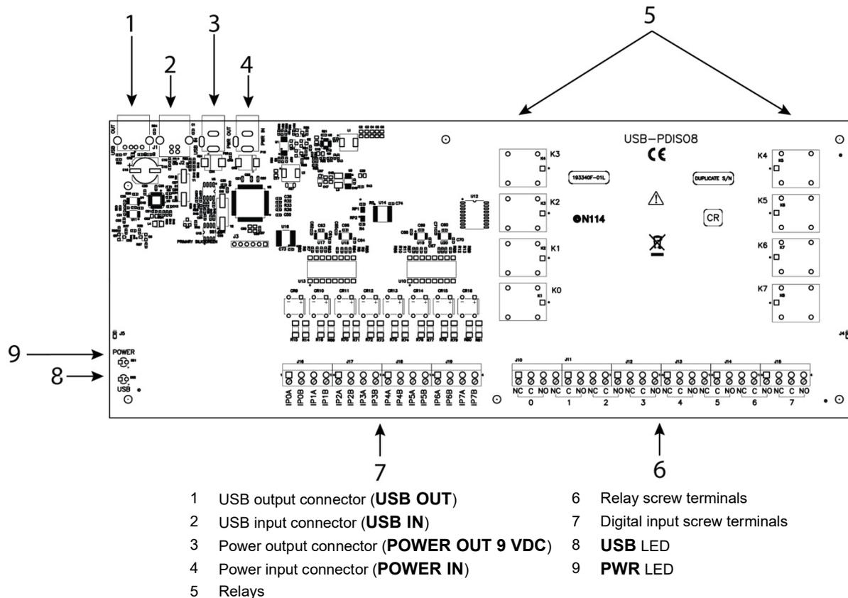
Figure 2. USB-PDISO8 components
