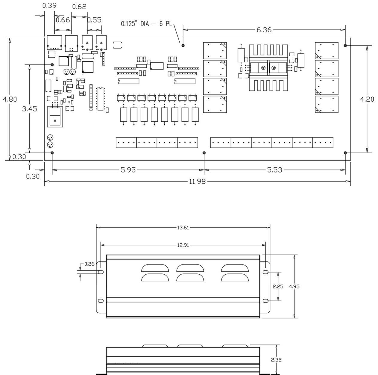
Figure 9. Circuit board (top) and housing dimensions
