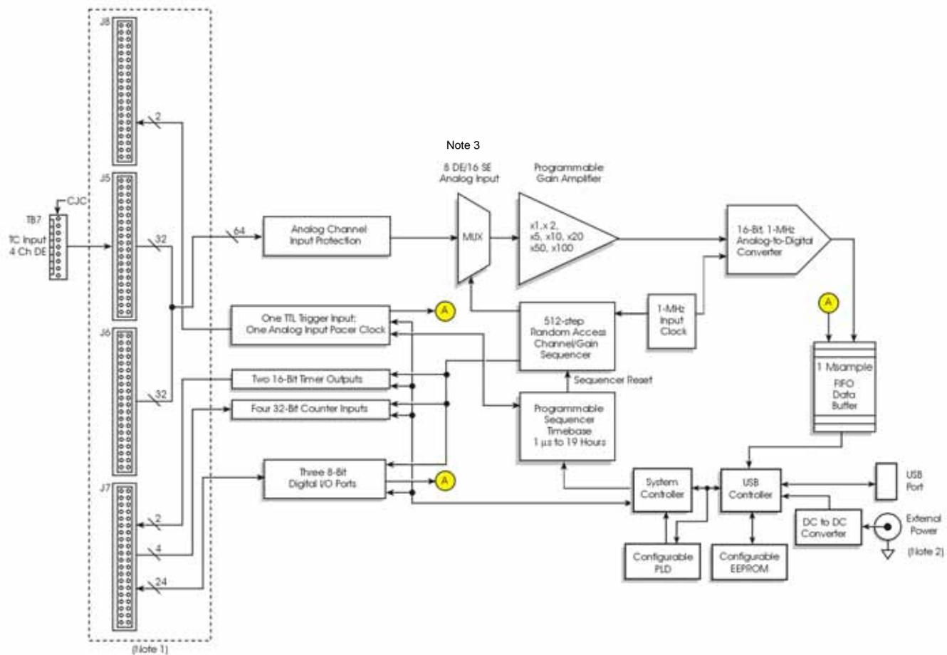
**Block Diagram for DaqBoard/3005USB and /3035USB**
