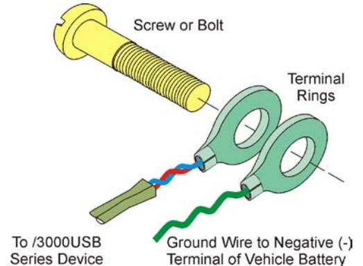
***Running a Ground Wire to the Battery's Negative Terminal***
