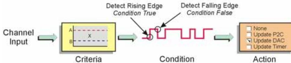
A digital detect signal is used to indicate when a signal condition is True or False, i.e., whether or not the signal has met the defined criteria. The detect signals themselves can be part of the scan group and can be measured as any other input channel; thus allowing real time data analysis during an acquisition.
