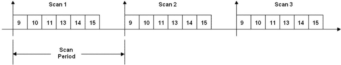
*DaqBoard/3000USB Series board Acquisition of Six Readings per Scan*
