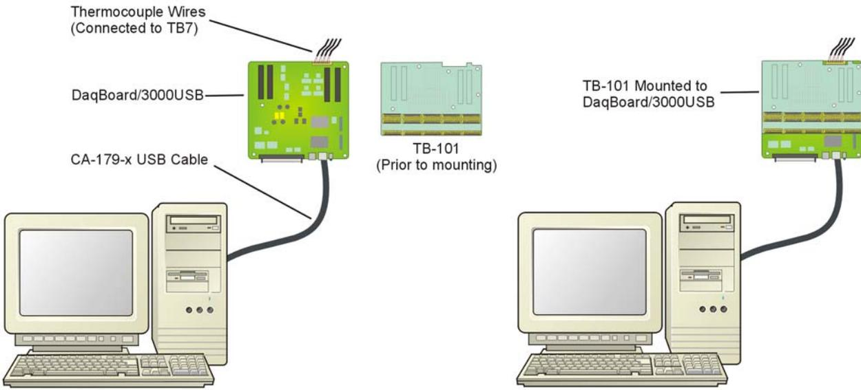
In this setup a TB-101 terminal board is plugged directly into the 40-pin headers (J5, J6, J7, and J8) of the main board. No cables are used in making this connection. “Stand-offs” are used to keep the boards from touching (instructions are provided on the following page).
