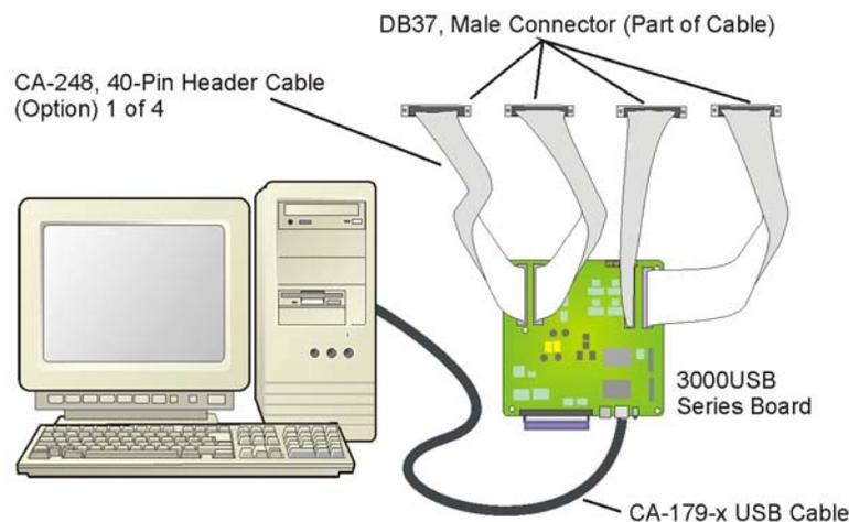
In this setup a CA-248 cable is connected to each of the 40-pin headers (J5, J6, J7, and J8). The result is four male DB37 connectors which, as can be seen from the pinouts, offer the same signal connectivity as the SCSI connector. Note that the J6 header is dedicated entirely to analog expansion and therefore is not applicable to /3001USB or /3005USB. As in all scenarios, a CA-179-x USB cable is used to connect the /3000USB Series board to a USB2.0 port on the host PC.
