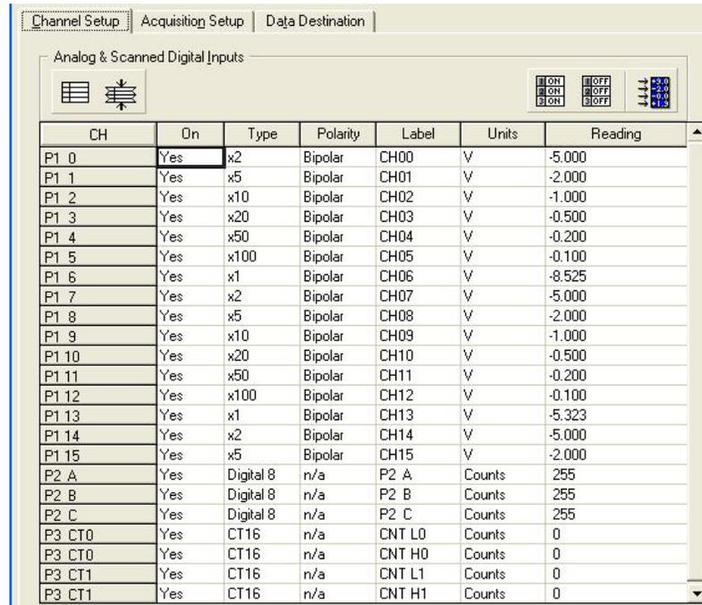
The screenshot shows the 'Channel Setup' window with the 'Analog & Scanned Digital Inputs' section. A table lists various channels with their status, gain, type, polarity, label, units, and current readings.
