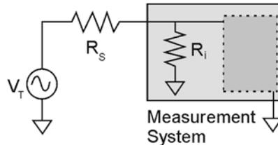
With input impedance ( $R_i$ ) of 10 M $\Omega$ , which is a realistic value for many measurement systems, a low source impedance ( $R_s$ ) of less than 100 $\Omega$  usually presents no problem. Signals from sources with impedance greater than 100 $\Omega$  should have appropriate signal conditioning.
