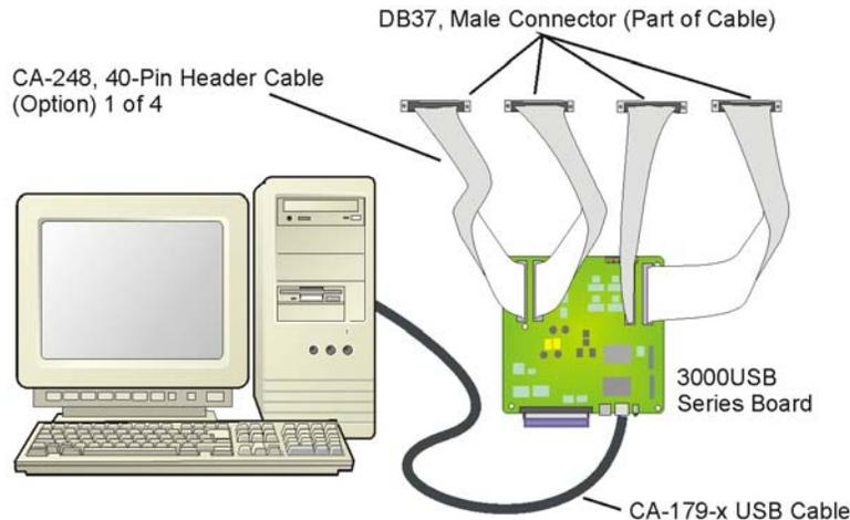
In this setup a CA-248 cable is connected to each of the 40-pin headers (J5, J6, J7, and J8). The result is four male DB37 connectors which, as can be seen from the pinouts, offer the same signal connectivity as the SCSI connector. Note that the J6 header is dedicated entirely to analog expansion and therefore is not applicable to /3001USB or /3005USB. As in all scenarios, a **CA-179-x USB cable is used to connect the /3000USB Series board to a USB port on the host PC.** USB2.0 is recommended.
