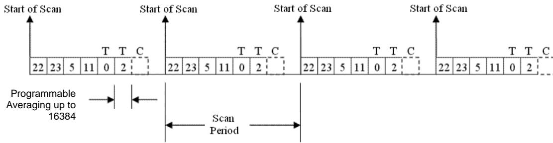
In this example, the desired number of oversamples is 256, therefore each analog channel in the scan group requires 256 microseconds to return one 16-bit value. The oversampling is also done for CJC temperature measurement channels. The minimum scan period for this example is therefore  $7 \times 256 \text{ us}$  or 1792 microseconds. The maximum scan frequency is the inverse of this number, 558 Hz.
