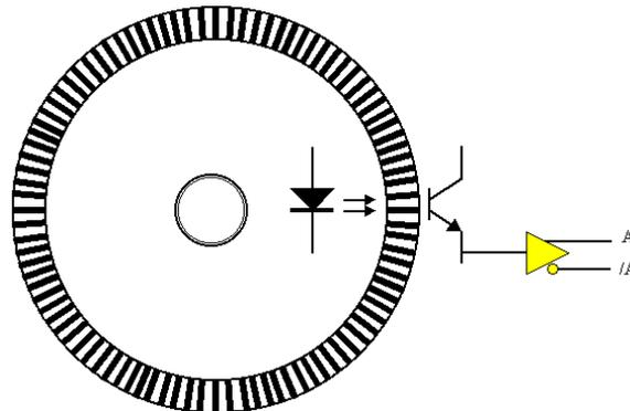
The concentric pattern for B has the same number of window pairs as A except that the entire pattern is rotated by 1/4 of a window-pair. Thus the B signal will always be 90 degrees out of phase from the A signal. The A and B signals will pulse 512 times (or 1024, 4096, etc.) per complete rotation of the encoder.
