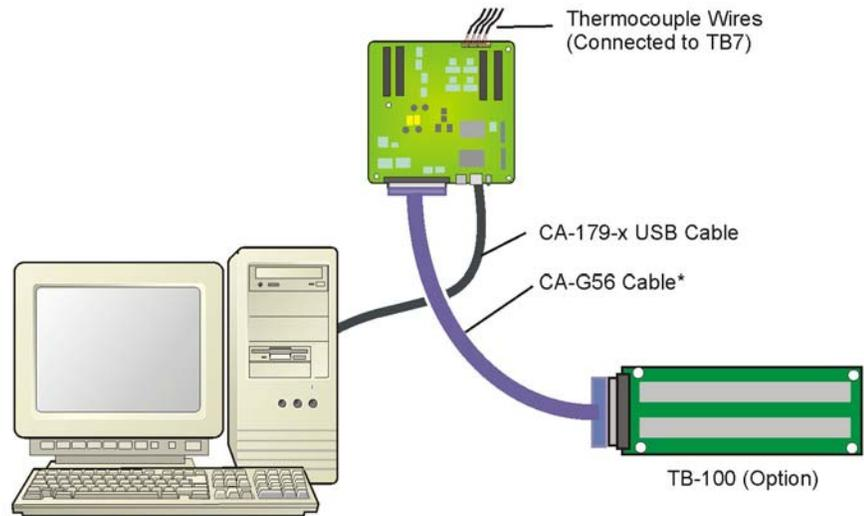
In this setup a TB-100 screw-terminal board option is connected to the 68-pin SCSI connector via a CA-G56 shielded cable. However, the use of other cables is possible as noted below. In this example we can also see that 4 thermocouples are connected at TB7 (on the /3000USB board). This means that 8 analog channels [to obtain 4 differential TC channels] are required (see following figure). Redundant connections must be avoided.
