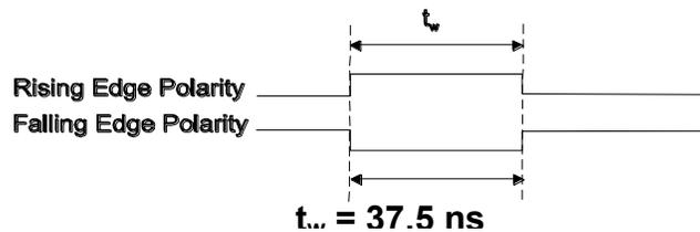
Figure 20. D/A CONVERT input signal timing
