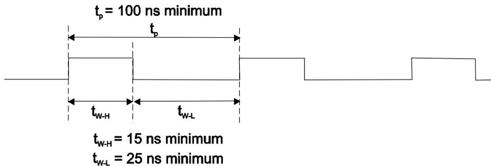
Figure 26. CTR2 CLK Signal Timing
