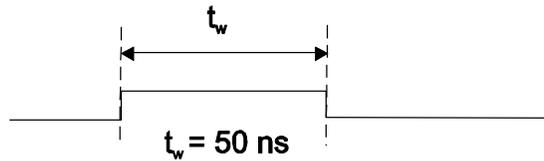
Figure 12. STARTSCAN start of scan timing
