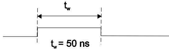
Figure 17. A/D STOP signal timing
