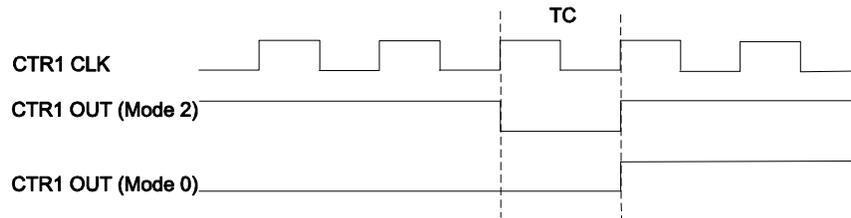
Figure 25. CTR1 OUT signal timing
