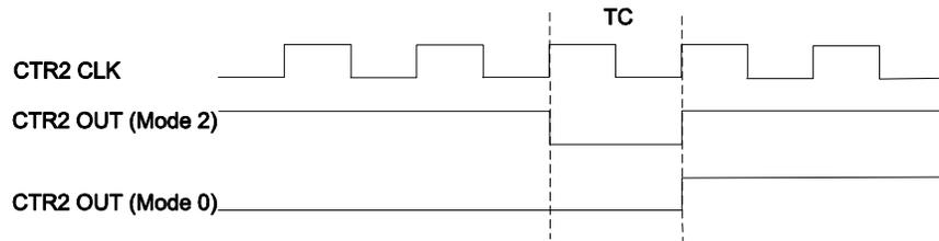
Figure 28. CTR2 OUT signal timing
