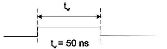
Figure 8. A/D START TRIGGER output signal timing
