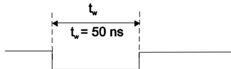
Figure 15. A/D CONVERT signal output timing requirement
