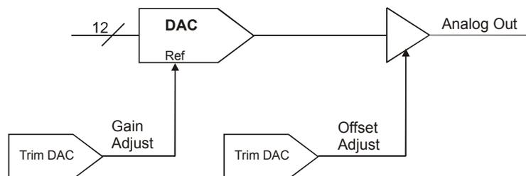
Figure 30. Analog output calibration
