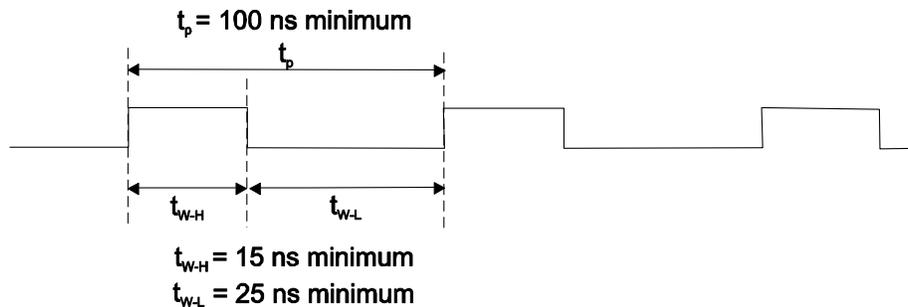
Figure 23. CTR1 CLK signal timing
