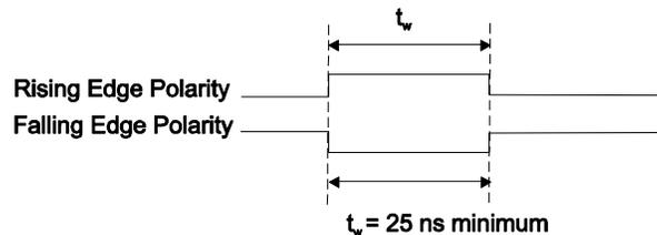
Figure 27. CTR2 GATE Signal Timing
