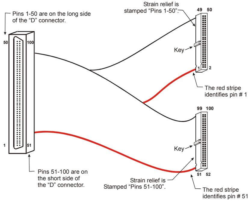
Figure 1. C100HD50-x cable connections
