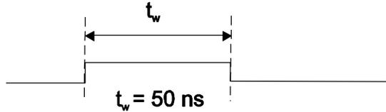
Figure 11. A/D STOP TRIGGER output signal timing
