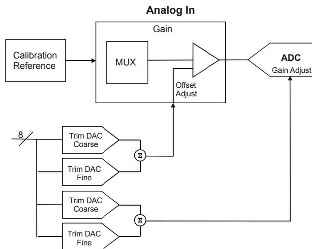
Figure 29. Analog input calibration
