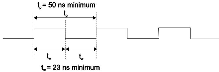
Figure 16. A/D EXTERNAL TIME BASE signal timing
