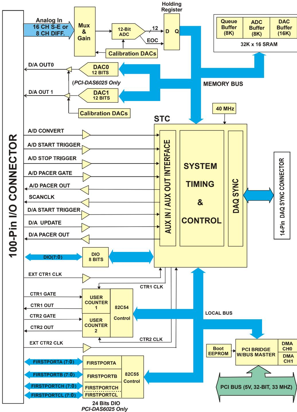
Figure 4. Block diagram – PCI-DAS6025 and PCI-DAS6023
