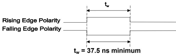
Figure 14. A/D CONVERT signal input timing requirement
