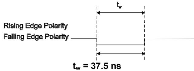
Figure 7. A/D START TRIGGER input signal timing
