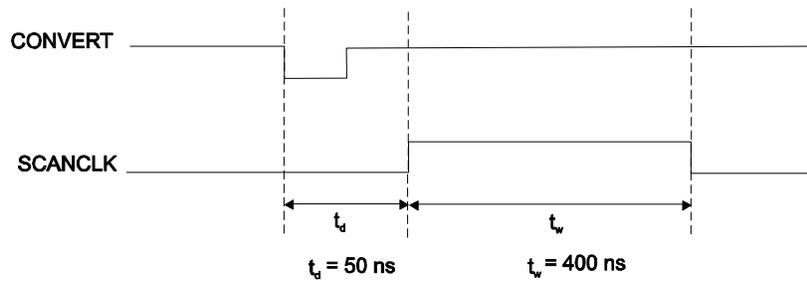
Figure 5. SCANCLK Signal Timing
