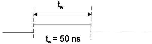
Figure 19. D/A START TRIGGER output signal timing
