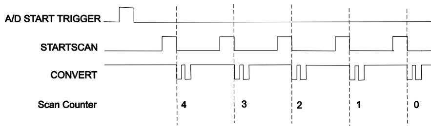
Figure 6. Data Acquisition Example for Conventional Triggering
