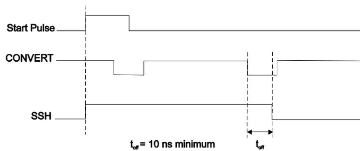
Figure 13. SSH signal timing
