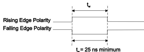
Figure 24. CTR1 GATE signal timing
