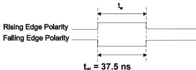
Figure 18. D/A START TRIGGER input signal timing
