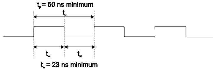
Figure 22. D/A EXTERNAL TIME BASE signal timing
