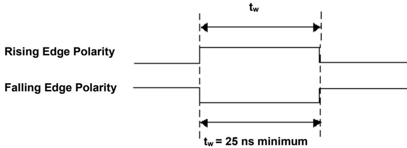
Figure 36. CTR2 GATE signal timing
