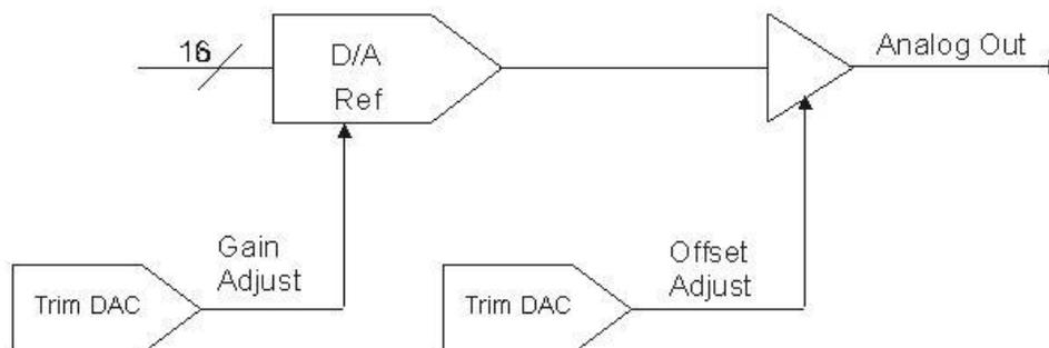
Figure 39. Analog output calibration – basic elements
