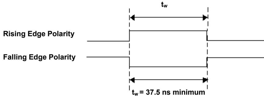
Figure 29. D/A CONVERT input signal timing
