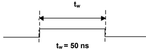
Figure 28. D/A START TRIGGER output signal timing
