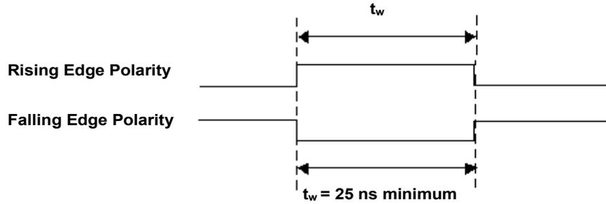
Figure 33. CTR1 GATE signal timing
