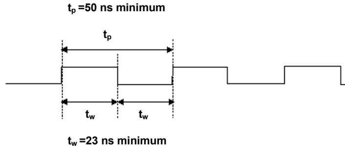
Figure 31. D/A EXTERNAL TIME BASE signal timing
