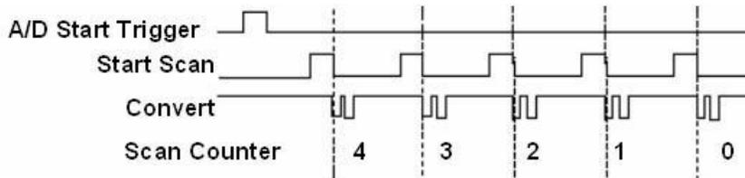
Figure 6. Data acquisition example for conventional triggering
