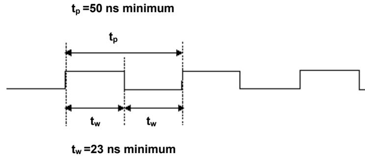
Figure 16. A/D EXTERNAL TIME BASE signal timing
