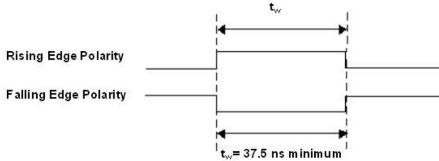
Figure 10. A/D STOP TRIGGER input signal timing
