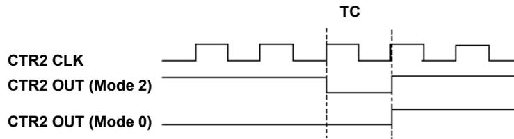
Figure 37. CTR2 OUT signal timing
