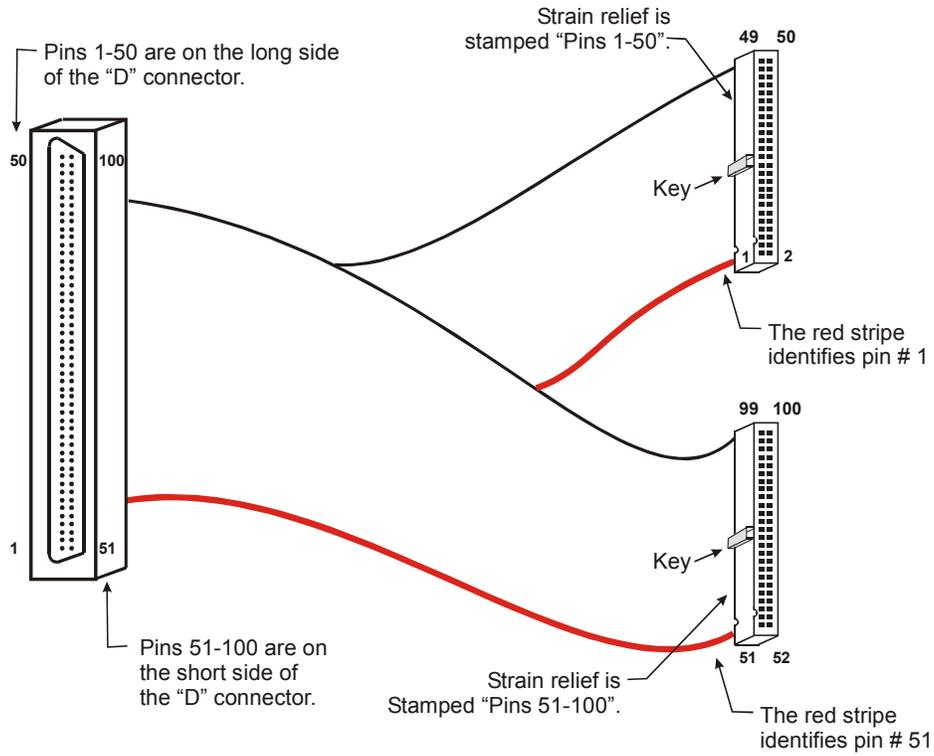
Figure 1. C100HD50-x cable connections
