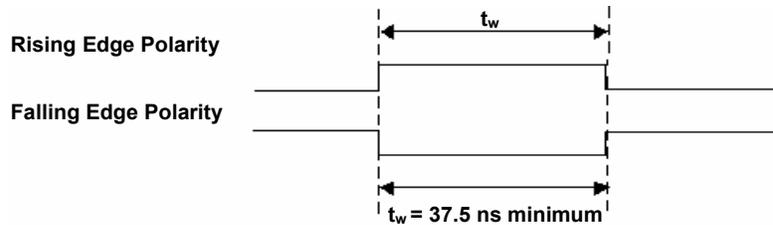
Figure 14. A/D CONVERT signal input timing requirement
