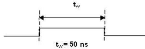
Figure 11. A/D STOP TRIGGER output signal timing
