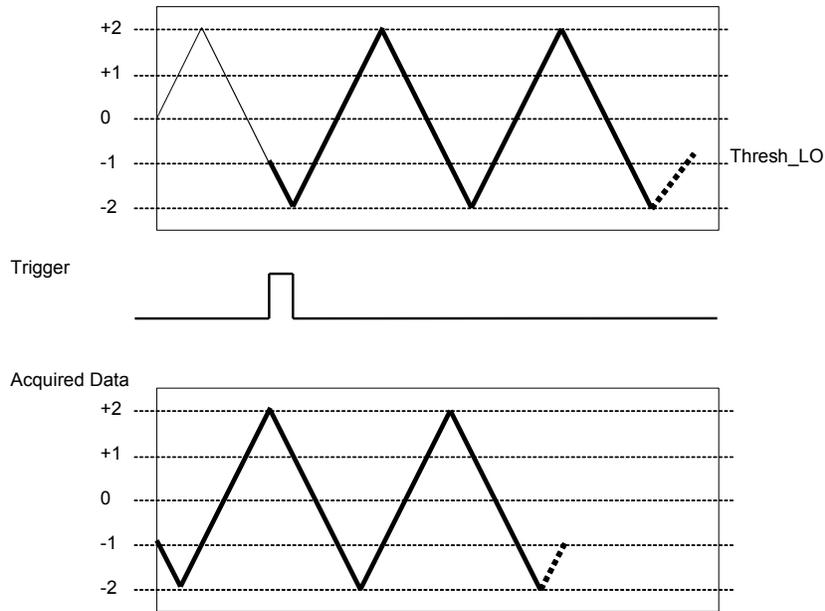
Figure 20. Trigger negative slope
