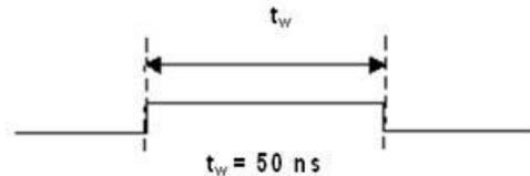
Figure 8. A/D START TRIGGER output signal timing
