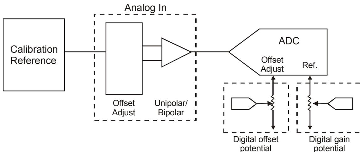
Figure 4-1. Analog input calibration
