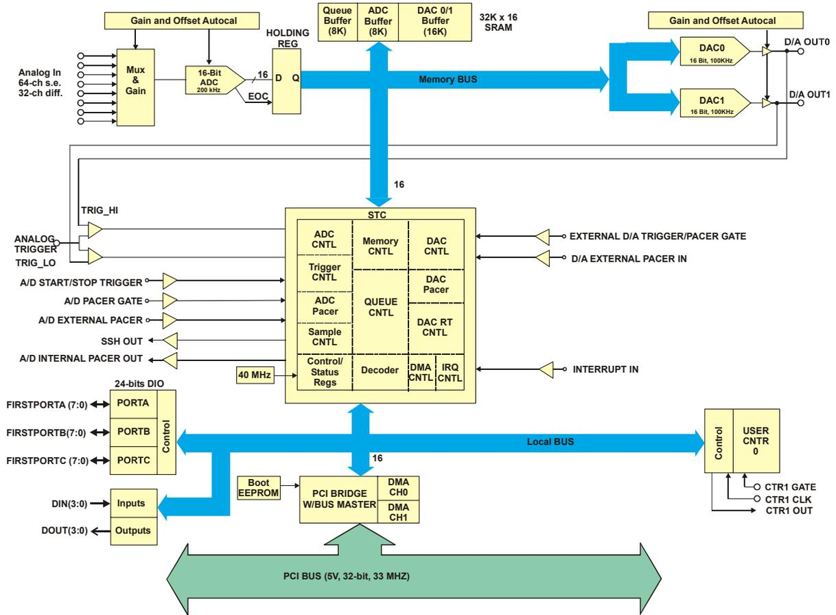
Figure 1-1. PCI-DAS6402/16 functional block diagram
