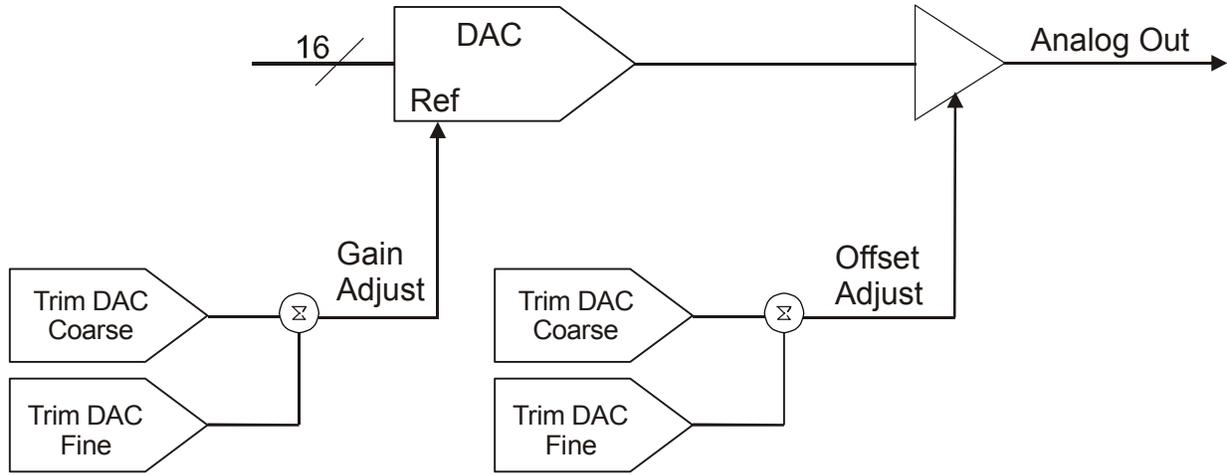
Figure 4-2. Analog output calibration
