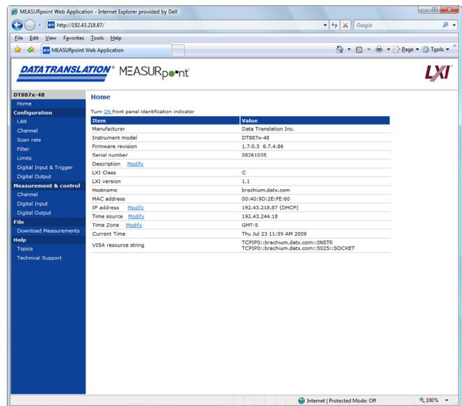
**The main web page displays information about your Ethernet instrument on the network and allows you to configure device settings.**
